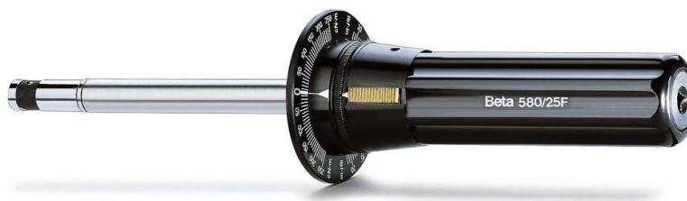
Figure 12. Torque measuring device: Beta 580/25F 1/4" Drive Dial Torque Screwdriver (Beta Utensili S.P.A, Sovico, Italy); 0 - 250 N-cm torque range with \pm 6\% torque accuracy for right-hand and left-hand tightening.
