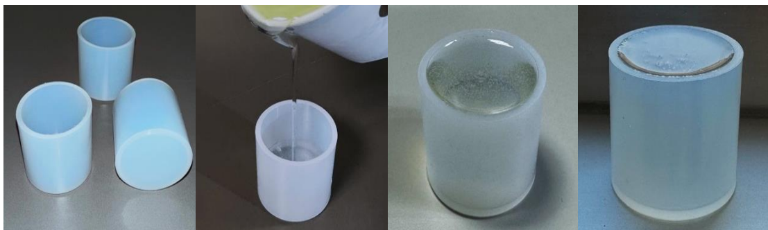
Figure (3.1): The preparation of the epoxy resin models into their molds.
