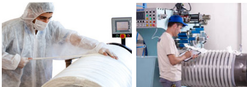
Figure 4.21 High voltage coils.
