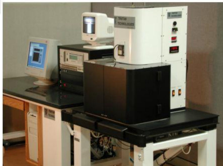
Figure 2.13. SQUID scanning microscope model SMM-770 with dc and ac biasing magnets.
