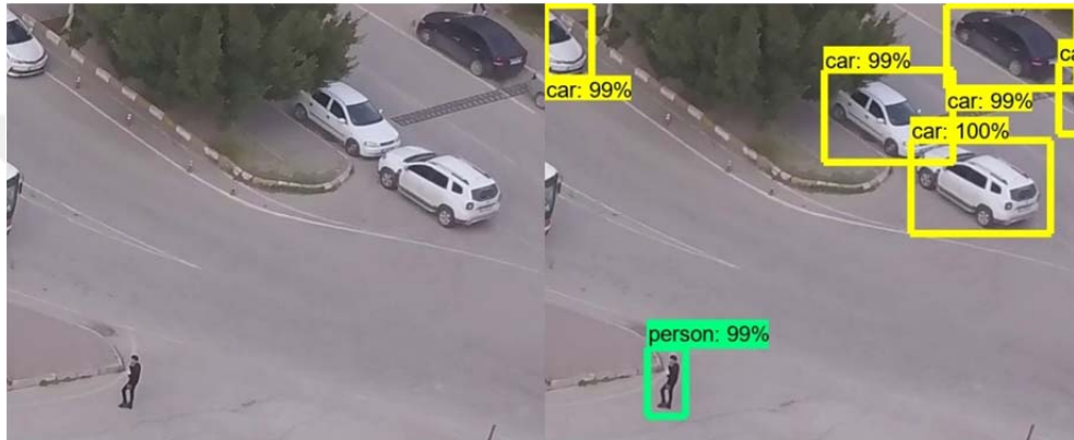
Figure 2.23. Output of the aerial images a walking person, and five cars with labels, and boundary boxes at 40 mt. altitude.
