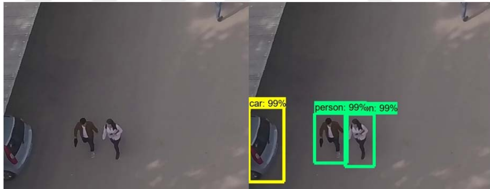
Figure 2.22. Output of the aerial images two walking person, and a car with labels, and boundary boxes at 20 mt. altitude.
