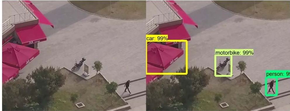
Figure 2.21. Detection of a motorbike, a walking person and a localization error of a car with labels, and boundary boxes at 30 mt. altitude.
