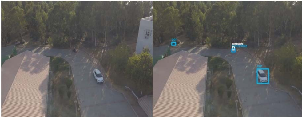
Figure 2.11. Output of the aerial images of two cars, and a person on a motorbike with labels, and boundary boxes at 15 mt. altitude.
