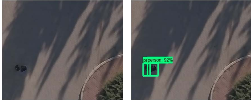
Figure 2.16. Output of the aerial images of two people with labels, and boundary boxes at 25 mt. altitude.
