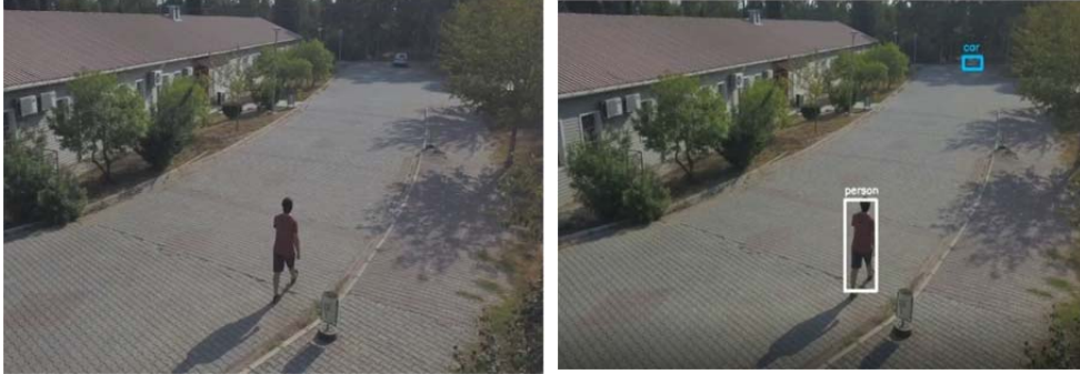
Figure 2.10. Output of the aerial images of a person, and a car with labels, and boundary boxes at 10 mt. altitude.
