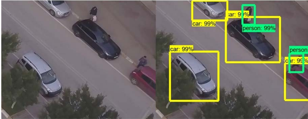
Figure 2.20. Detection of four cars, and two walking persons with labels, and boundary boxes at 30 mt. altitude.
