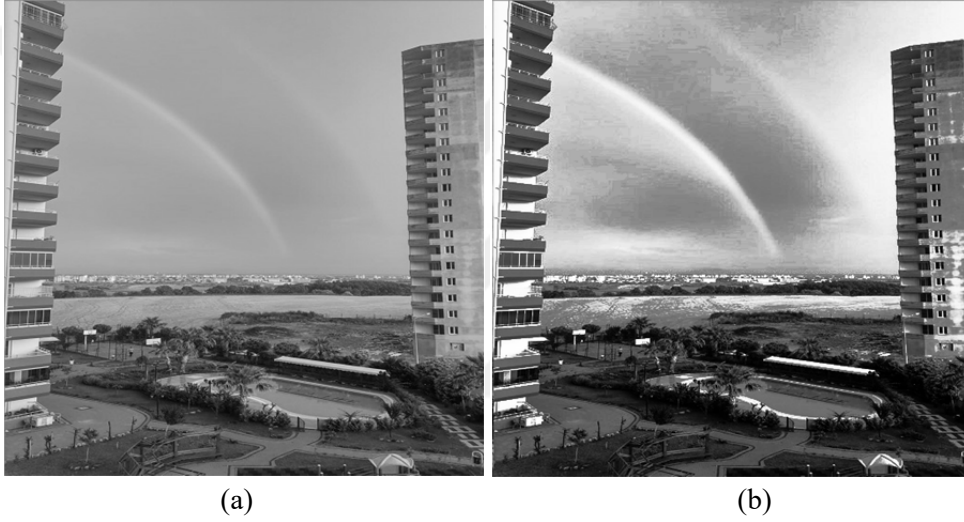
Figure 1.10. (a) original grayscale image, (b) after histogram equalization.
