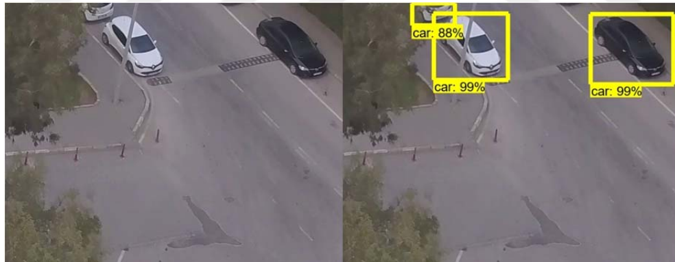
Figure 2.17. Output of the aerial images of three cars with labels, and boundary boxes at 25 mt. altitude.
