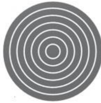
Figure 8: An annular array. There are 7 elements in this array.
