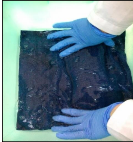
Figure 3.8 Micro-cracking coagulation bath
