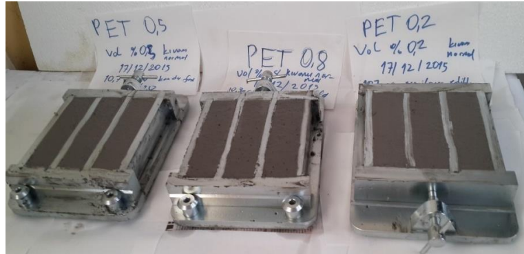
Figure 2.14 Sample of mortar prisms (Personal archive, 2017)
