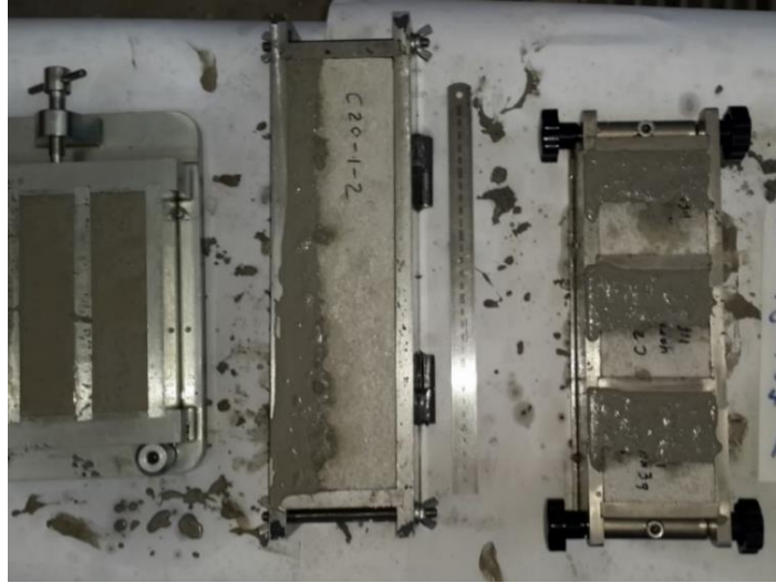
Figure 2.19 Repaired specimens at the 28 th day (Personal archive, 2017)
