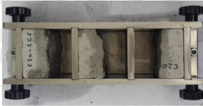
Figure 2.20 Tensile split resultant cube specimens before repairing (Personal archive, 2017)
