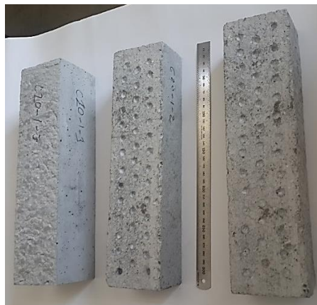
Figure 2.18 1 st group's 3 drilled beam specimens at the 28 th day (Personal archive, 2017)
