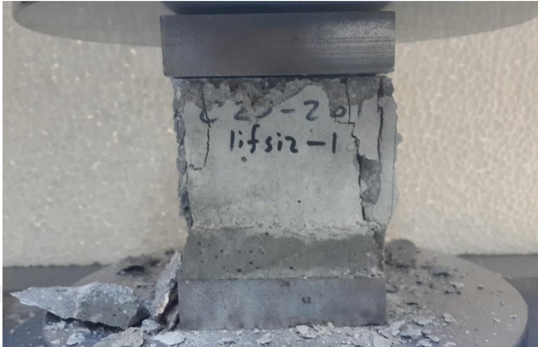
Figure 3.55 Failed SCM repaired concrete specimen under compression test (Personal archive, 2017)
