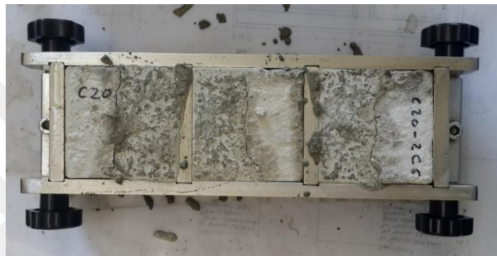
Figure 2.23 Cube specimens at the 29 th day after repaired and set (Personal archive, 2017)
