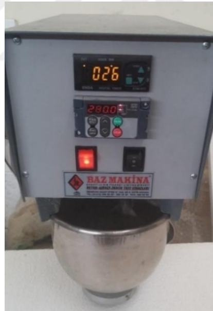
Figure 2.13 5-liter capacity mixer (Personal archive, 2017)
