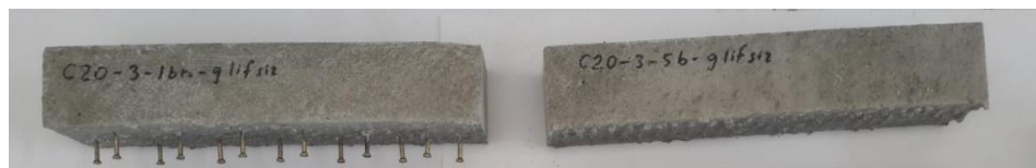
Figure 2.24 Nailed and surface-roughened specimens after 24 hours from casting (Personal archive, 2017)
