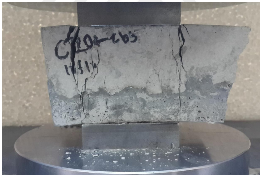
Figure 3.56 Failed PP- reinforced SCM repaired specimen under comp. test (Personal archive, 2017)
