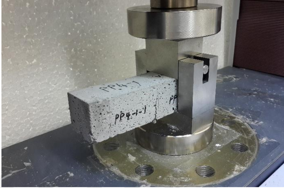
Figure 2.28 Mortar sample failed by compression test (Personal archive, 2016)
