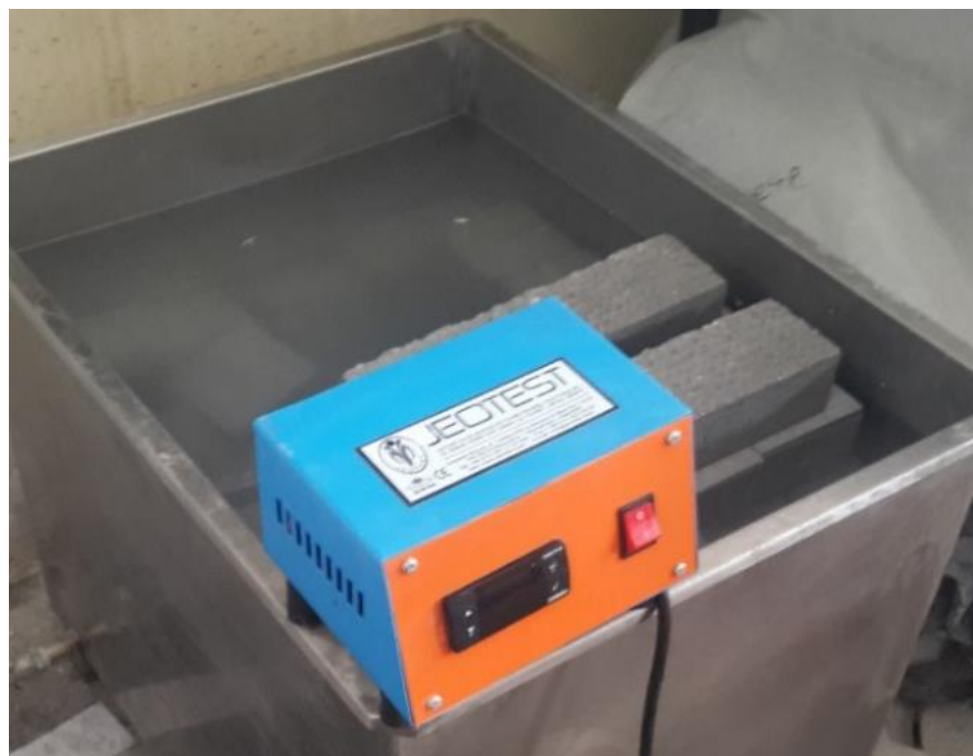
Figure 2.16 Curing tank (Personal archive, 2017)
