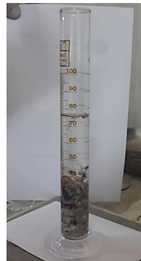
Figure 2.8 Density measurement (Personal archive, 2016)
