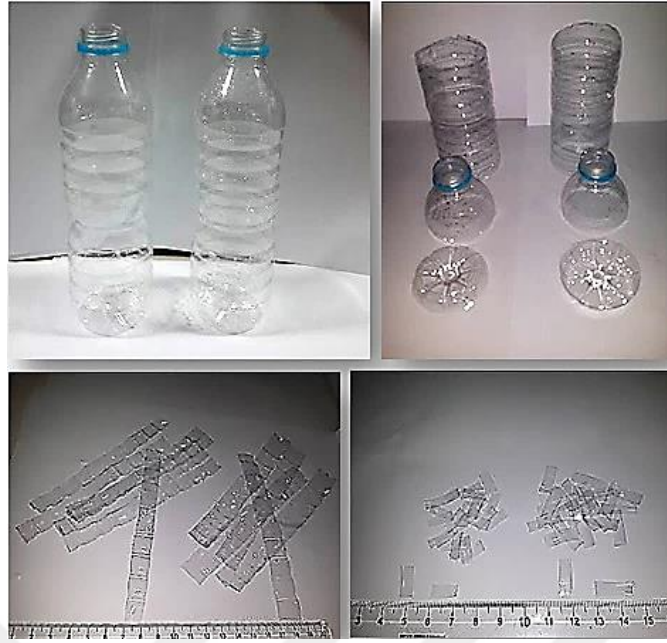
Figure 2.4 Cutting process of the used PET waste plastic fibers (Personal archive, 2016)
