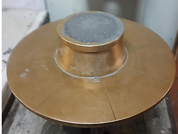
Figure 2.10 Mortar flow test apparatus (Personal archive, 2017)
