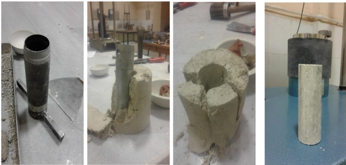
Figure 3.8. Unconfined compressive strength test sample preparation.
