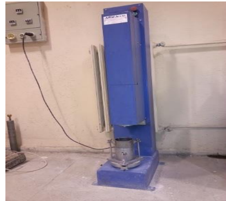
Figure 3.11. a). Standard proctor test mold with base plate b).electrical standard Proctor test machine.
