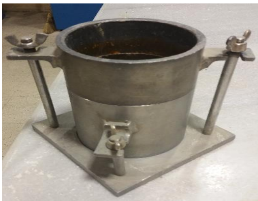
Figure 3.11. a). Standard proctor test mold with base plate b).electrical standard Proctor test machine.
