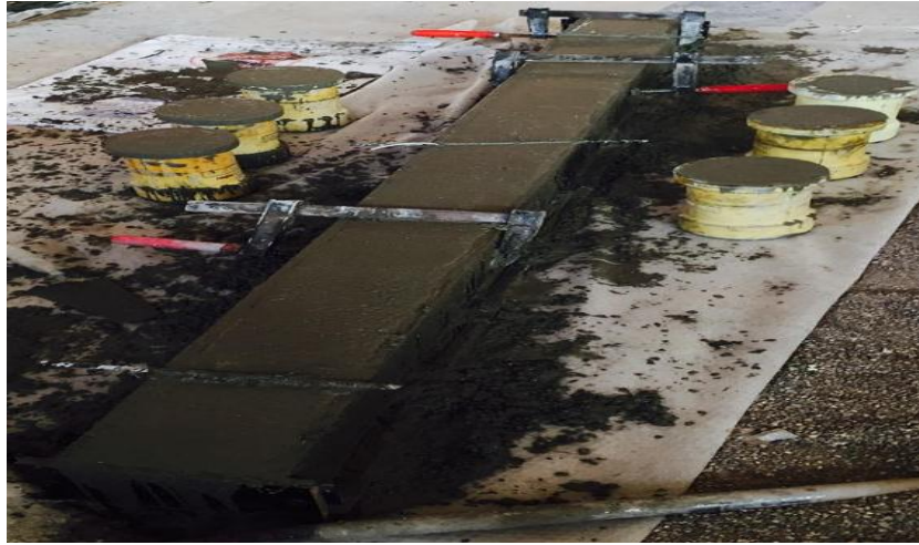
Figure 3.12 Final casting and vibrating stage.
