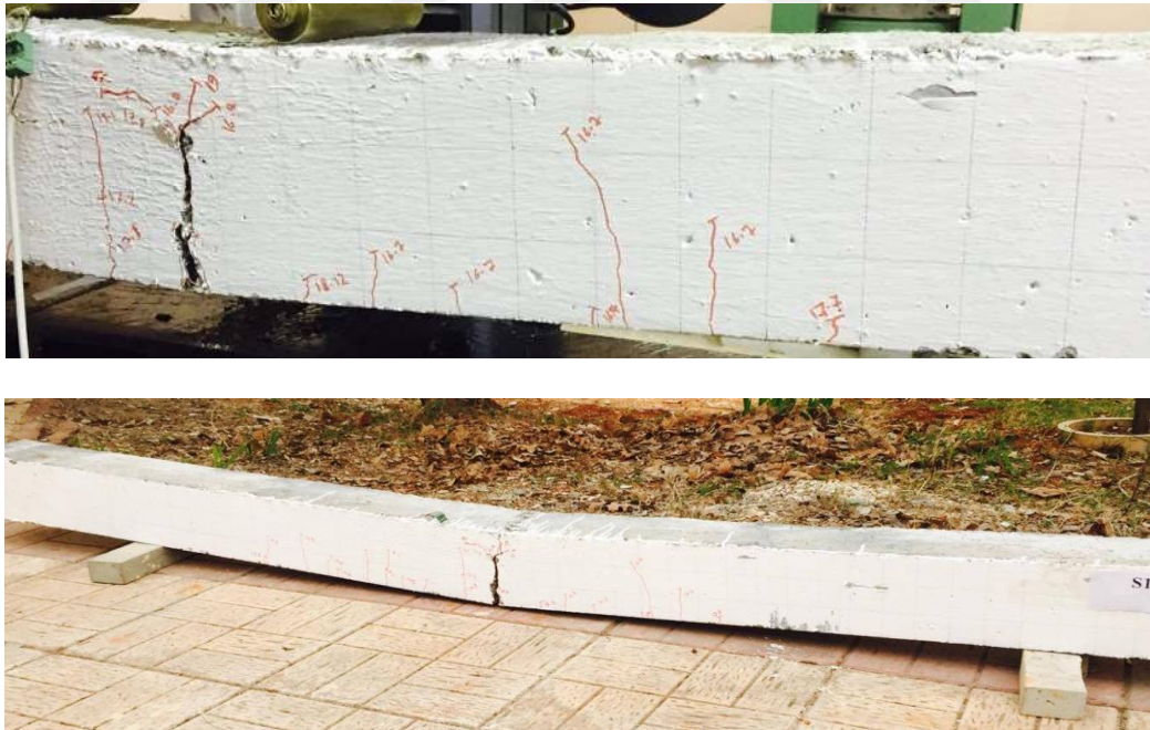
Figure 4.14 Structural failure of beam specimen S1-L8-0-3.
