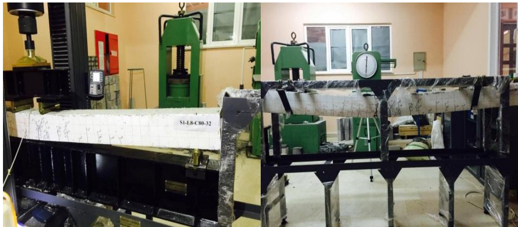
Figure 4.24 Structural failure for beam specimens of Group C.
