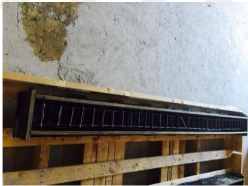
Figure 3.7 Fabrication of specimens with stirrups.
