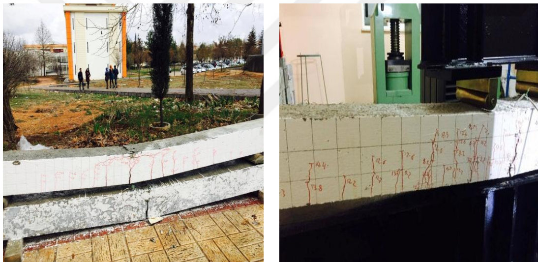
Figure 4.10 Structural failure of beam specimen N-L8-0-3.
