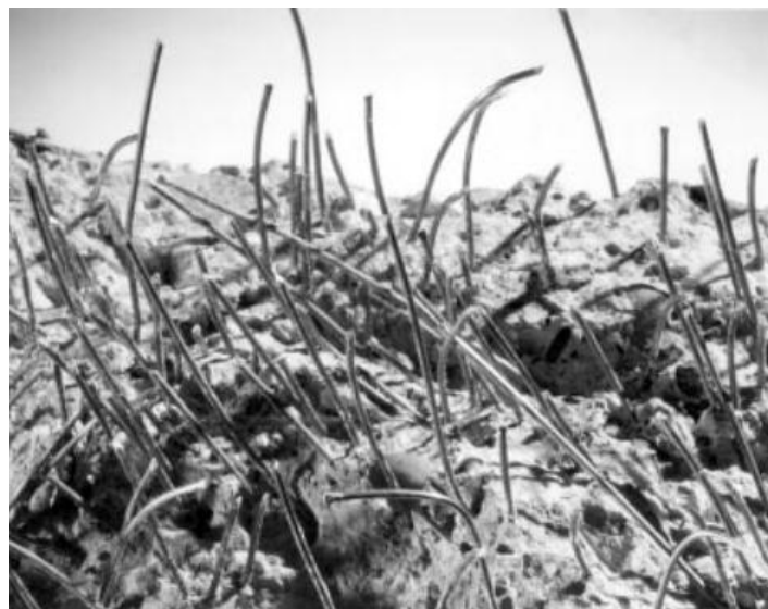
Figure 2.2 Fracture Surface of SFRC[26]
