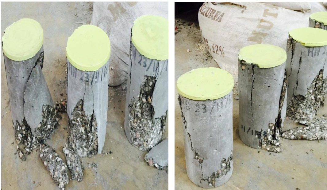
Figure 4.5 Failed cylindrical specimens in compressive test for the present study.
