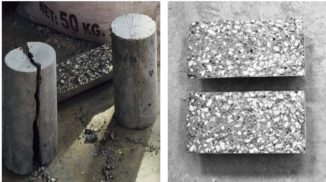
Figure 4.7 Failed cylindrical specimens in indirect tensile test for the present study.
