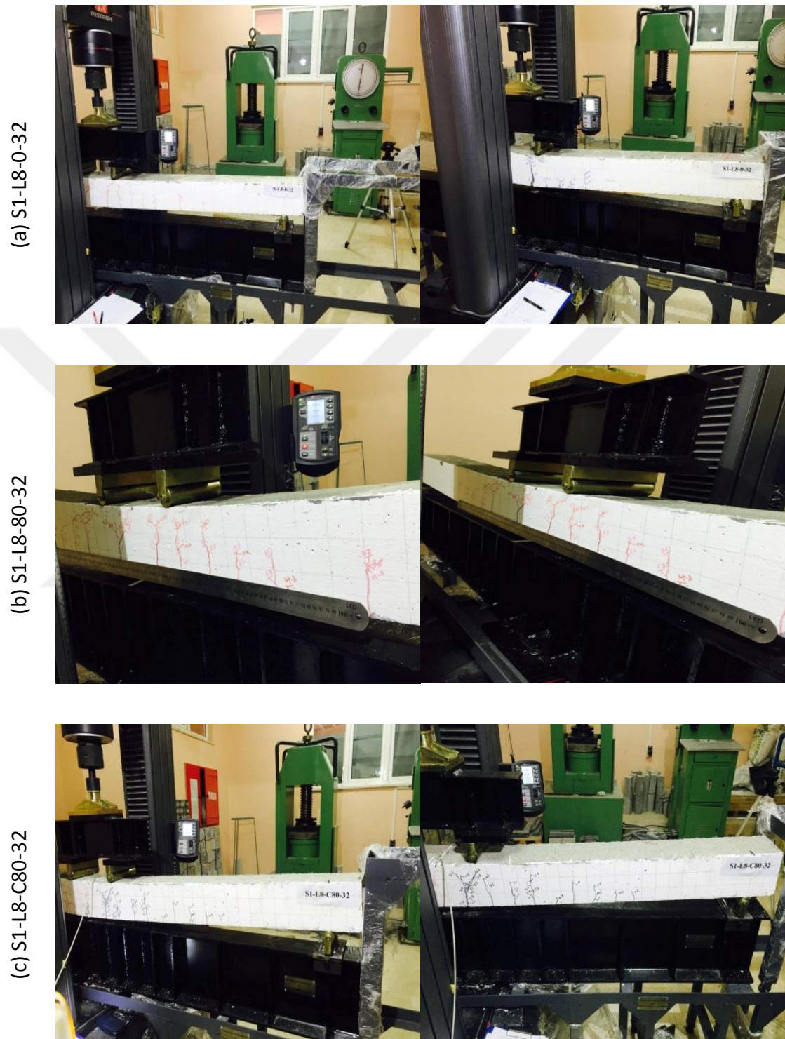
Figure 4.23 Crack pattern for beam specimens of Group C.
