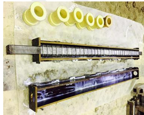
Figure 3.7 Fabrication of specimens with stirrups.
