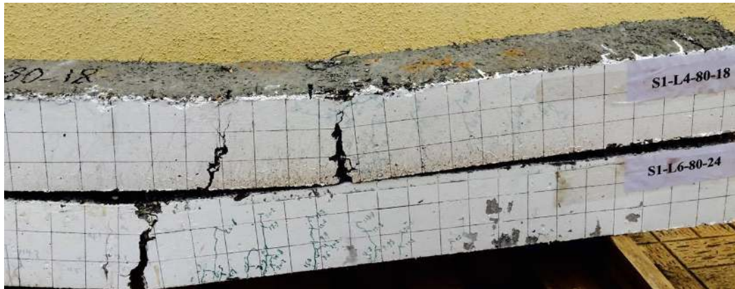
Figure 4.30 Structural failure for beam specimens S1-L6-80-24 and S1-L4-80-18.
