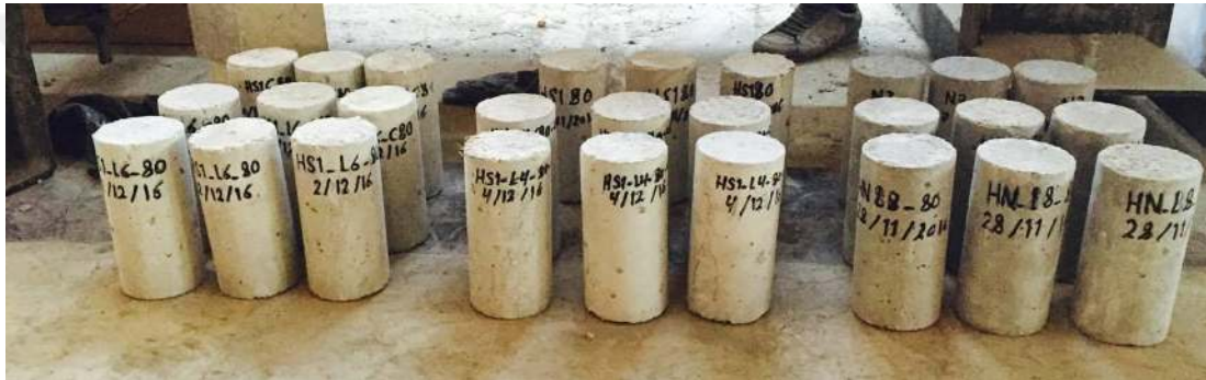
Figure 4.2 Cylindrical specimens fabricated in the present study.
