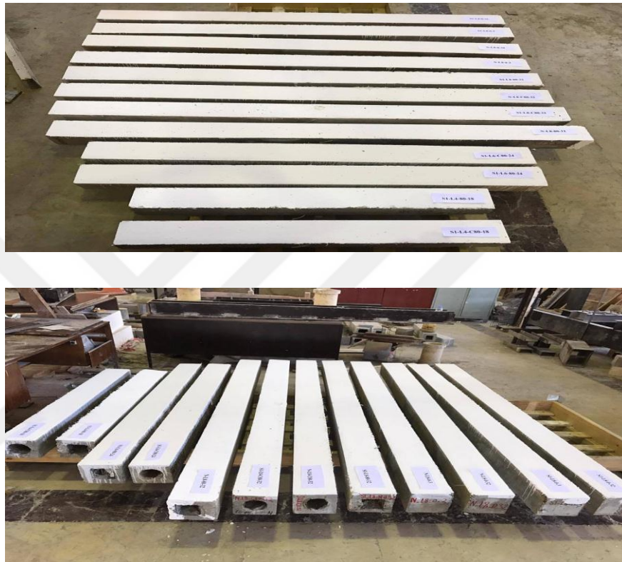
Figure 3.19 painting and meshing process of beam specimens
