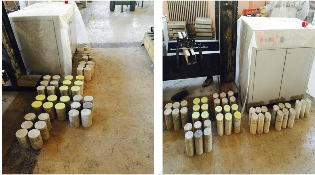
Figure 4.3 Sulfur capping of cylindrical specimens used in the present study.
