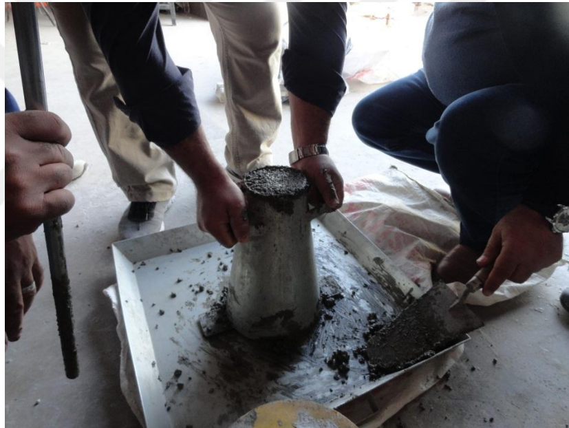
Figure 3.16 Slump test measurement.
