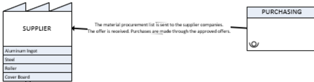
Figure 3.20 Information flow from purchasing unit to supplier
