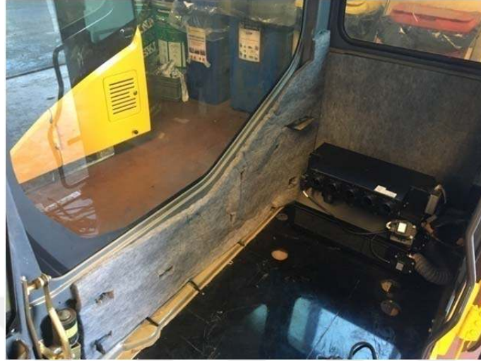
Figure 4.28. Visualization of Finished Cabin Carcass with Isolation
