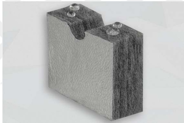
Figure 4.7. Cross Section of Oil and Water Repellent Polyester
