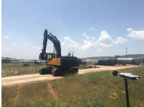
Figure 5.4. Figure in the Test Moment When Receiving Sound Values from Points Specified on the Vehicle
