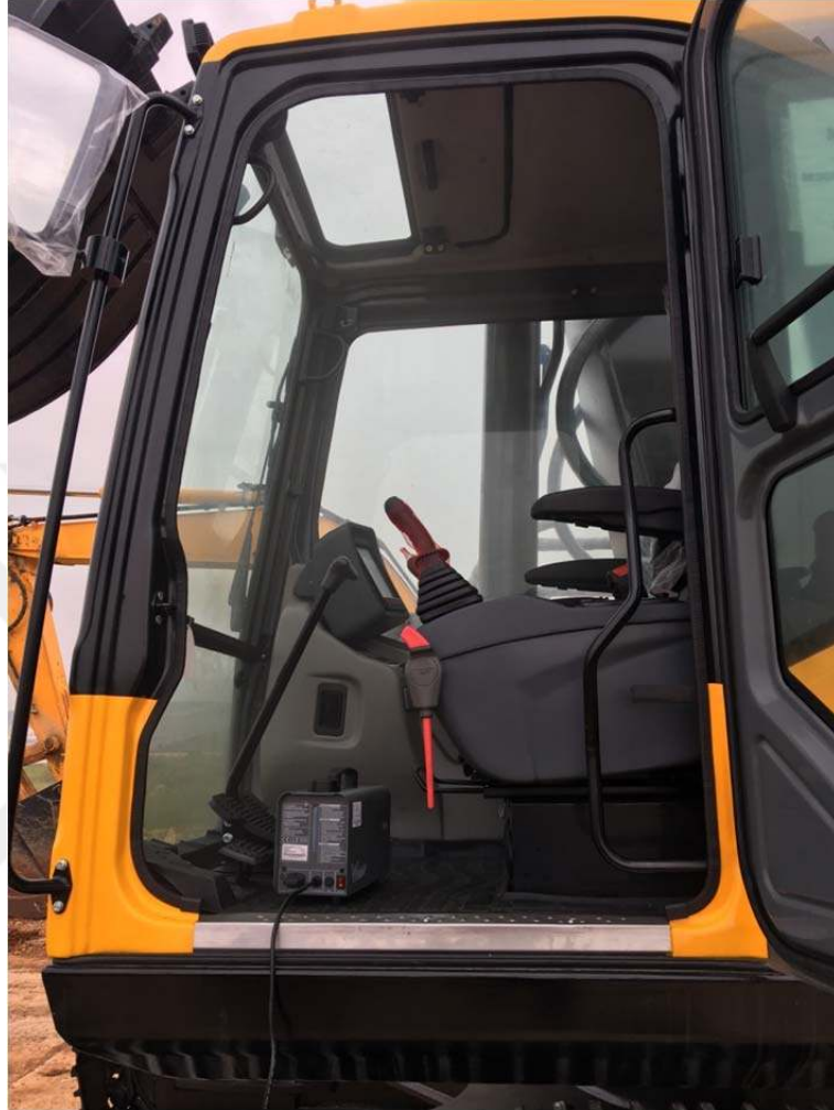
Figure 4.16. Test Equipment Installation for Excavator Cabin Fog Test
