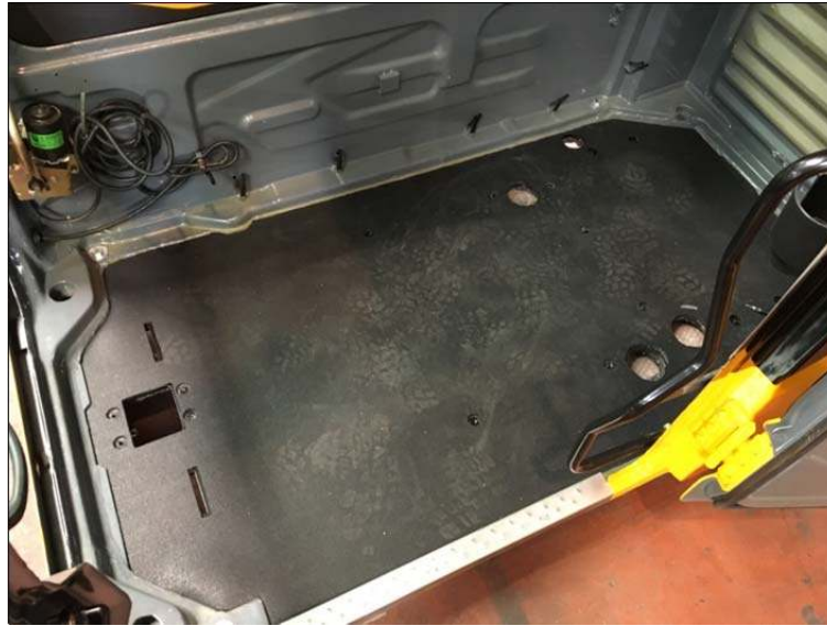
Figure 4.26. Mounting of Cabinet Base Outer Sound Absorber.
