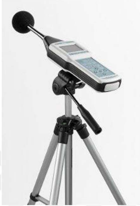
Figure 4.13. Delta Ohm UD-2010 Sound Level Meter
