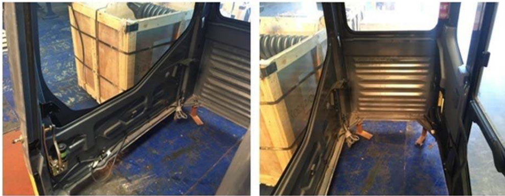
Figure 4.27. Polyester Insulation Coating Unfinished Cabin Carcass Visual
