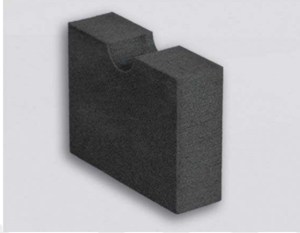
Figure 4.11. Cross Section of Cross-Linked Polyethylene Foam
