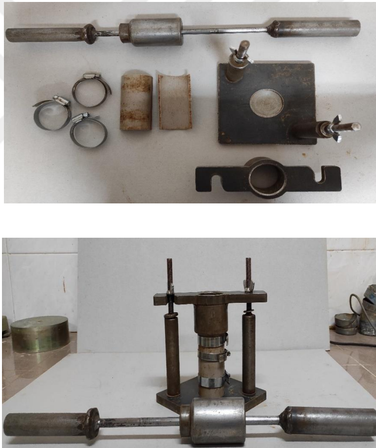
Figure 3.19. Unconfined compression test (UCS) apparatus and setup
