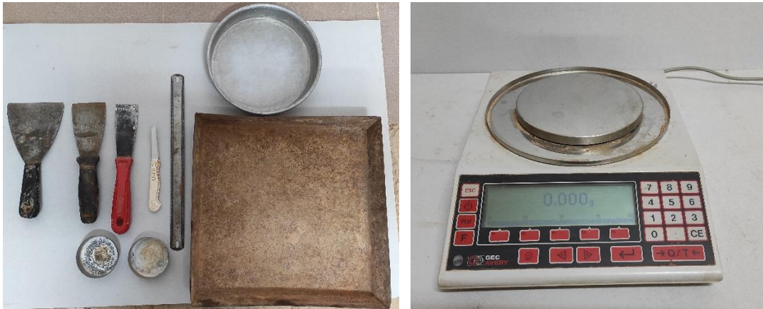
Figure 3.8. Apparatus and scale used to mix materials
