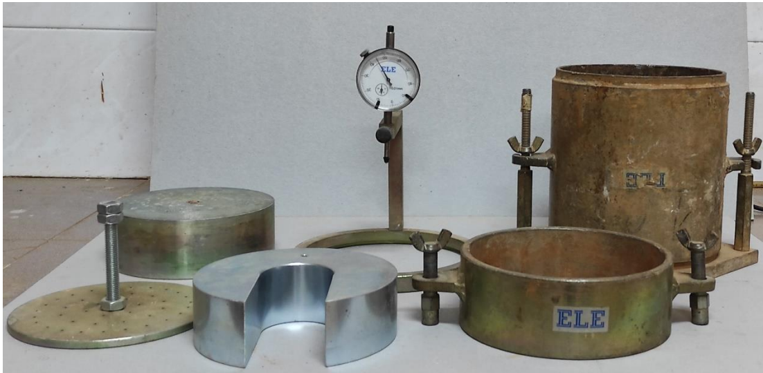
Figure 3.16. California bearing ratio (CBR) test apparatus
