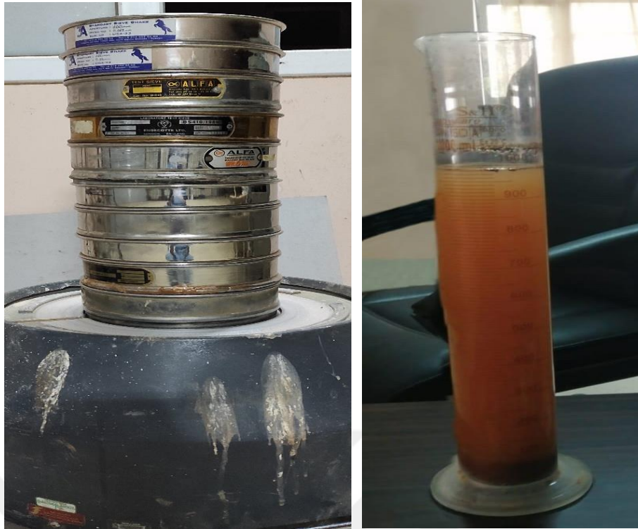
Figure 3.9. Sieve with sieve shaker and hydrometer
