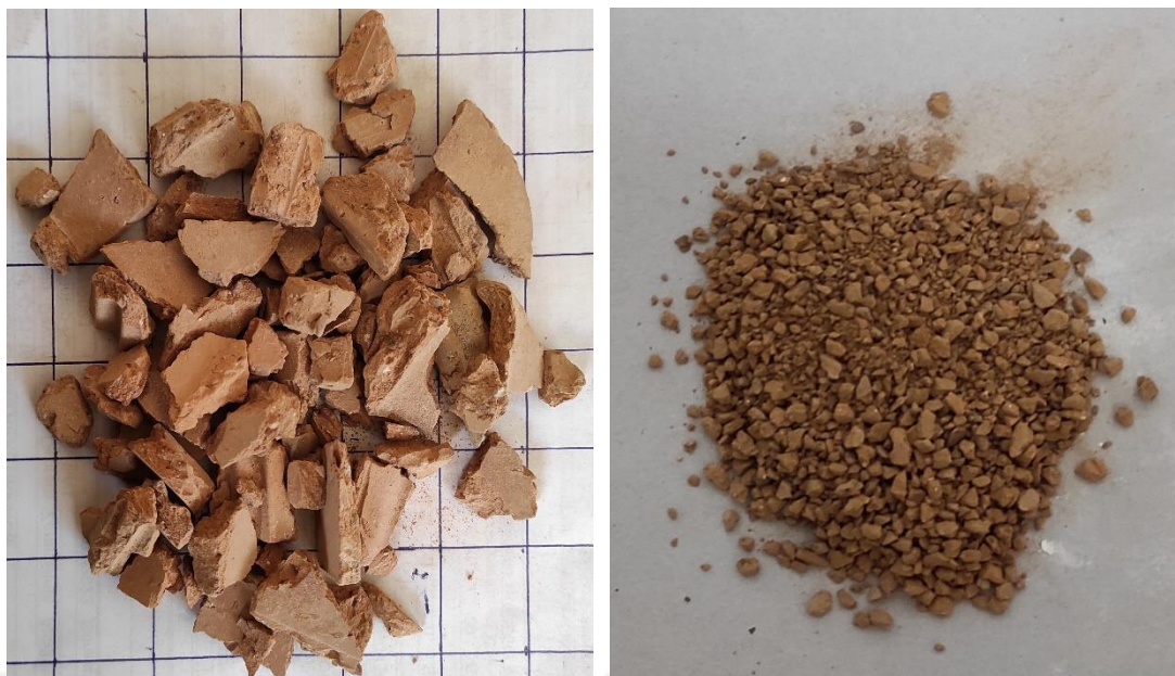
Figure 3.3. Photo of waste brick before and after breaking for experiments
