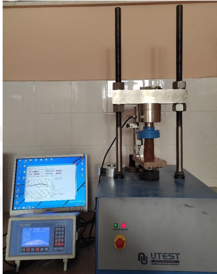
Figure 3.20. Unconfined compression tester during UCS sample testing
