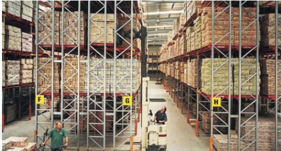
Figure 2.16 Double deep rack systems
