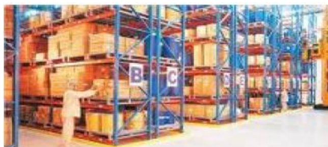
Figure 2.15 Back-to-back rack systems
