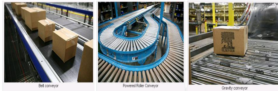
Figure 2.14 Belt roller and gravity conveyor (Trusty, 2014)
