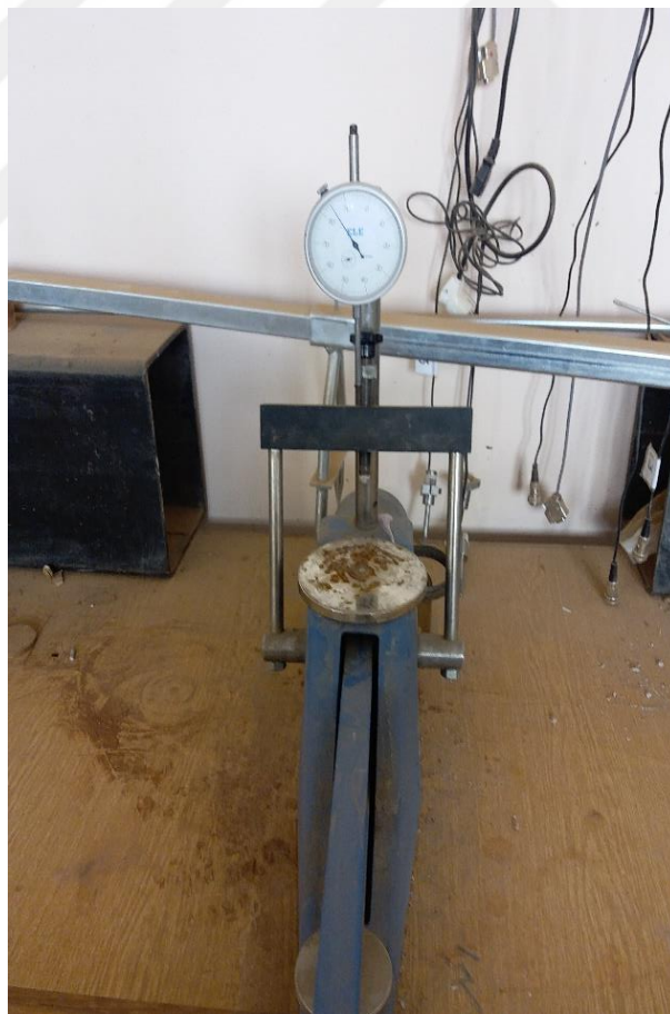
Figure 3.15 ELE consolidometer apparatus test device used during the test
