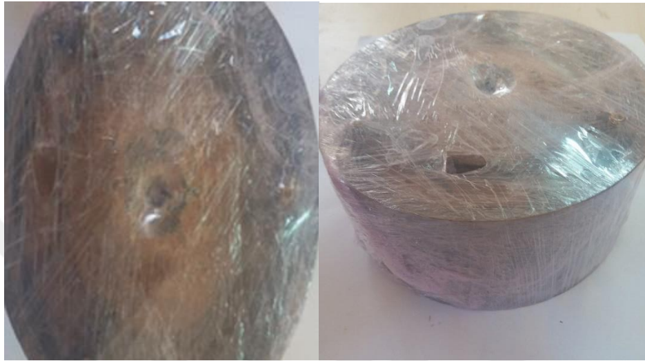
Figure 3.17 Sample before test with covering to prevent humidity
