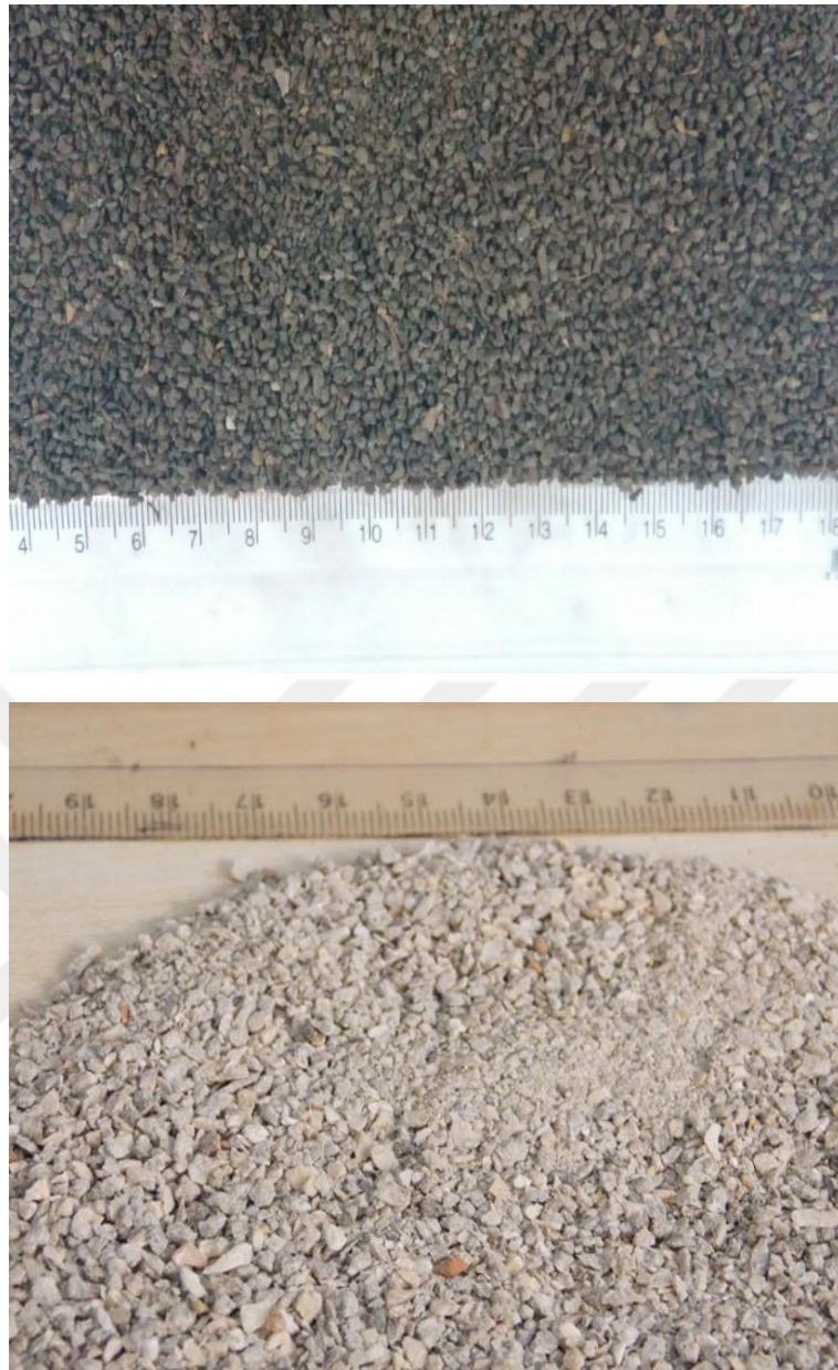
Figure 3.13 Pictures of organic soil and CWC size used in odometer test
