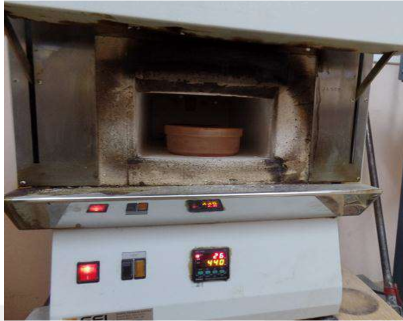
Figure 3.13 Muffle furnace with organic soil sample (Ibrahim, 2018).
