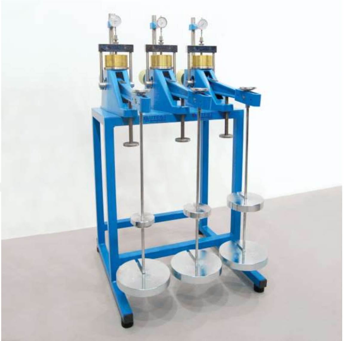
Figure 3.20 Consolidation test device used during experiment.
