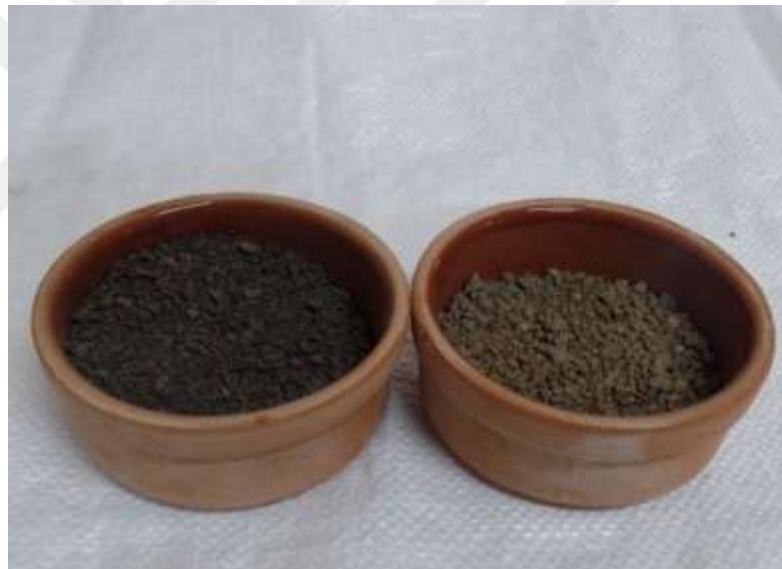
Figure 3.14 Organic soil samples (1) before oven (2) after oven (Ibrahim, 2018).
