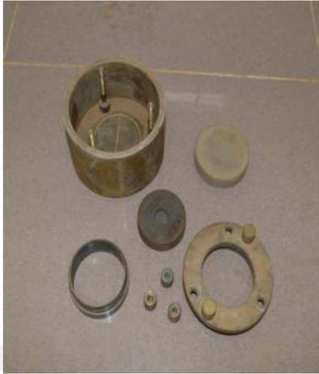
Figure 3.19 Apparatus of one-dimensional consolidation test.
