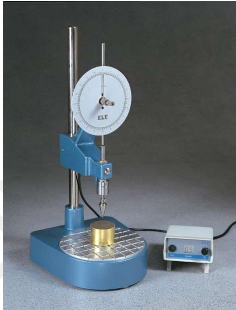
Figure 3.15 The fall cone apparatus during the test.
