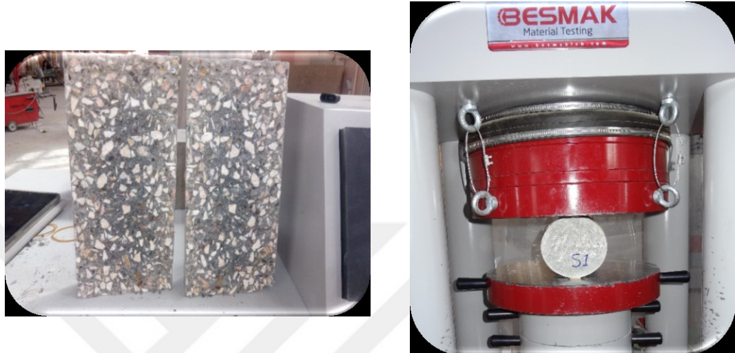
Figure 4.8 Tensile strength specimen
