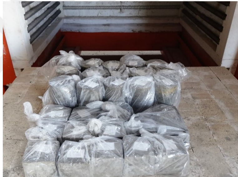
Figure 3.8 Curing samples by heating
