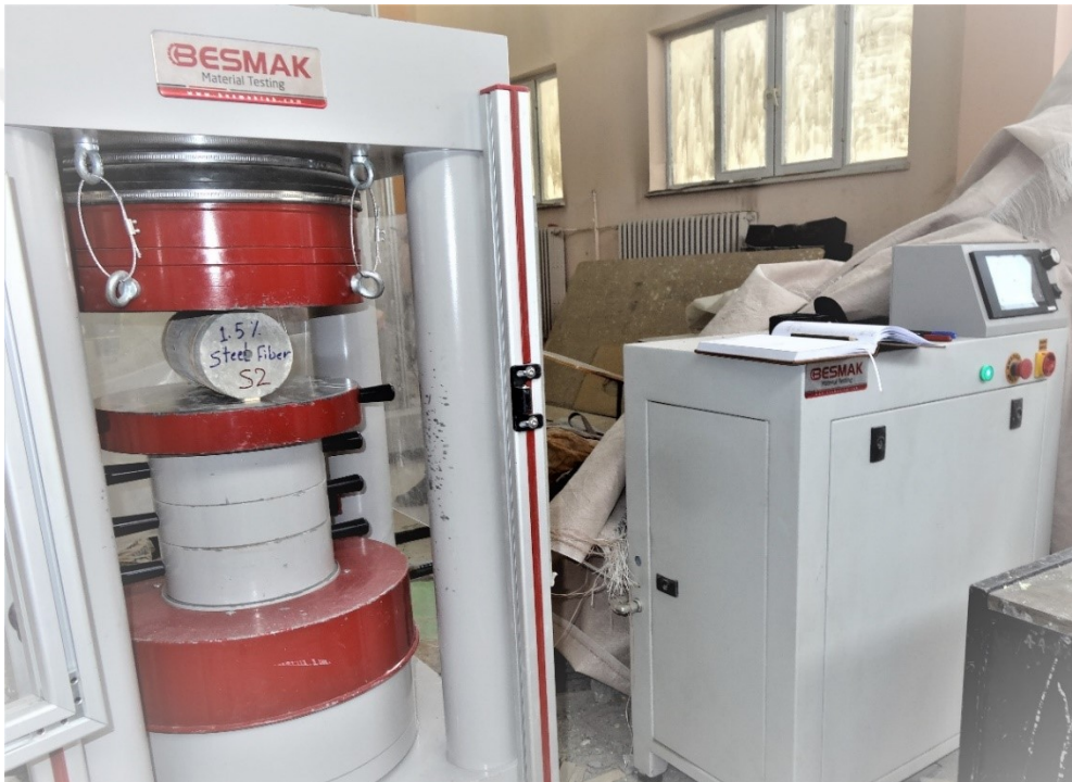
Figure 3.14 Photograph of the tensile test
