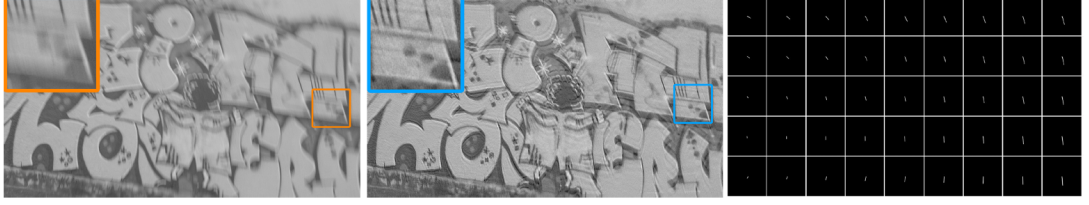
Figure 1.2: (Left) A real-world image with spatially-variant motion blur. (Center) Deblurred image with constant mesh-sized deblurring method. (Right) Blur kernels calculated from IMU motion estimates [6].
