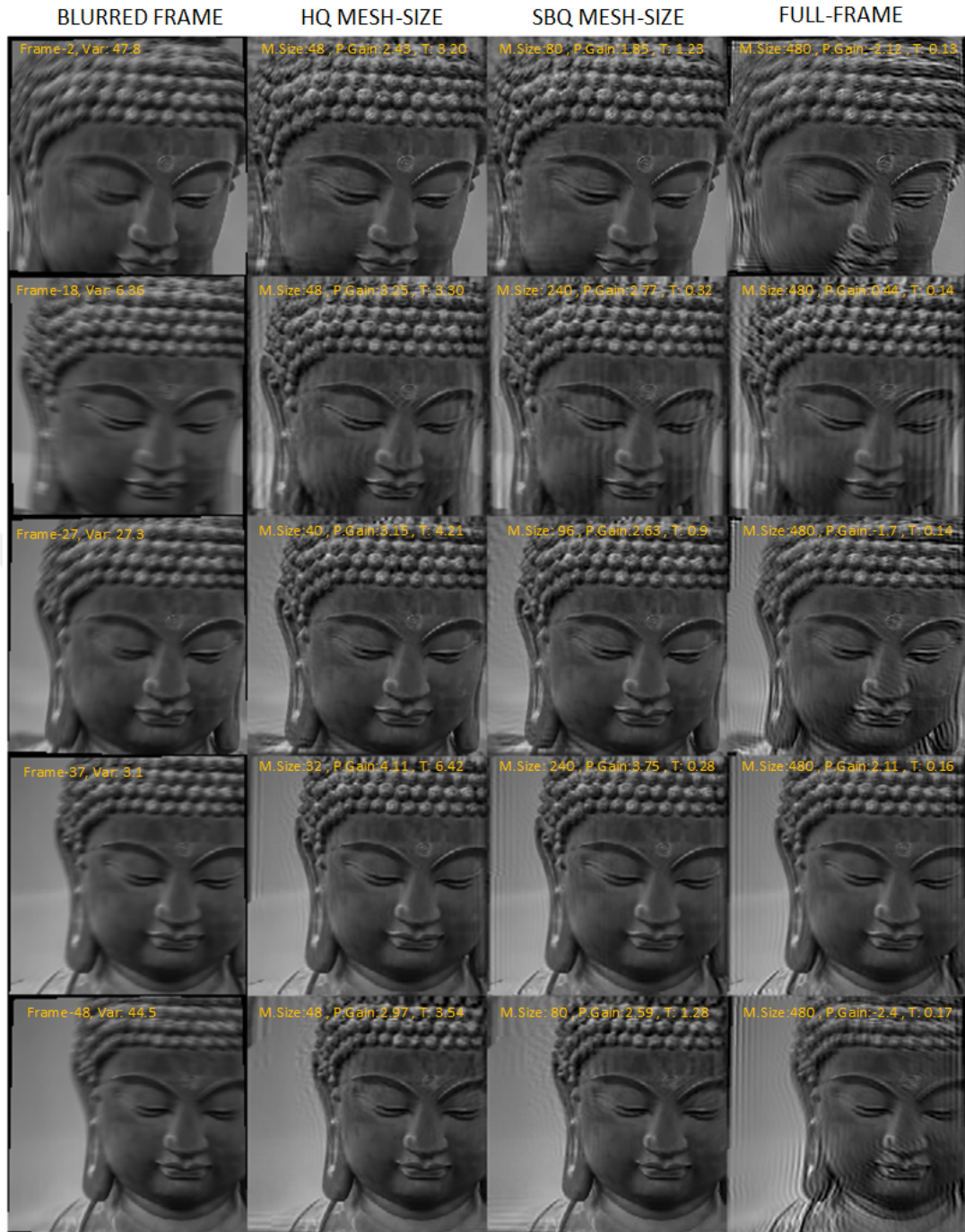
Figure 4.10: Shows blurred and deblurred frames with different mesh-sizes from Dataset-3. The mesh-size is represented as ‘M.size’, PSNR-Gain in dB as ‘P.Gain’, and computation time in sec as ‘T’. As mesh-size increases, the quality of deblurring and computation time decreases while decreasing mesh-size results in high quality and cost. The best quality is obtained in the HQ method and decreases from left to right except for frames with low variance.
