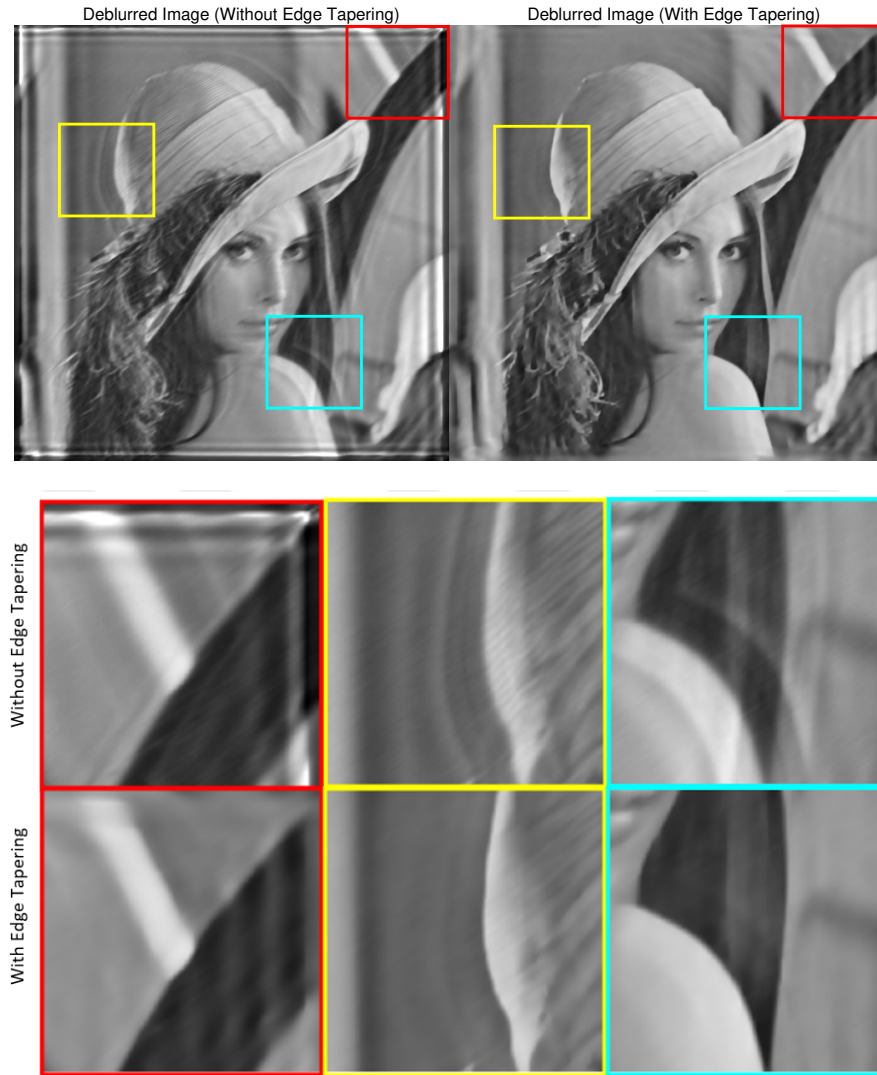
Figure 3.7: Shows the deblurred image results with and without edge tapering at the top figure. The selected boxes are magnified and the decrease in the ringing artifacts can be seen in results.
