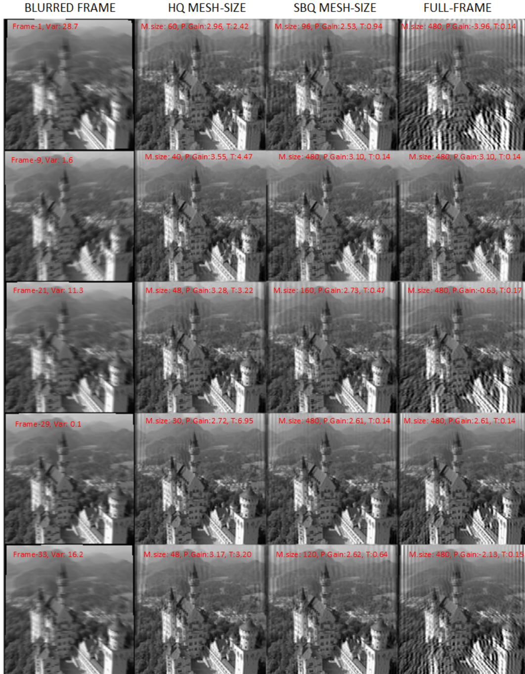
Figure 4.11: Shows blurred and deblurred frames with different mesh-sizes from Dataset-4. The mesh-size is represented as ‘M.size’, PSNR-Gain in dB as ‘P.Gain’, and computation time in sec as ‘T’. As mesh-size increases, the quality of deblurring and computation time decreases while decreasing mesh-size results in high quality and cost. The best quality is obtained in the HQ method and decreases from left to right except for frames with low variance.
