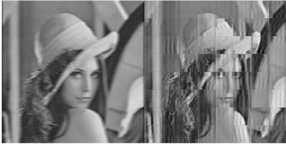
Figure 3.8: Shows the blurred image and deblurred image with mesh-grid size of [60x60] pixels respectively. The mesh-grid artifacts appear on each grid's border.
