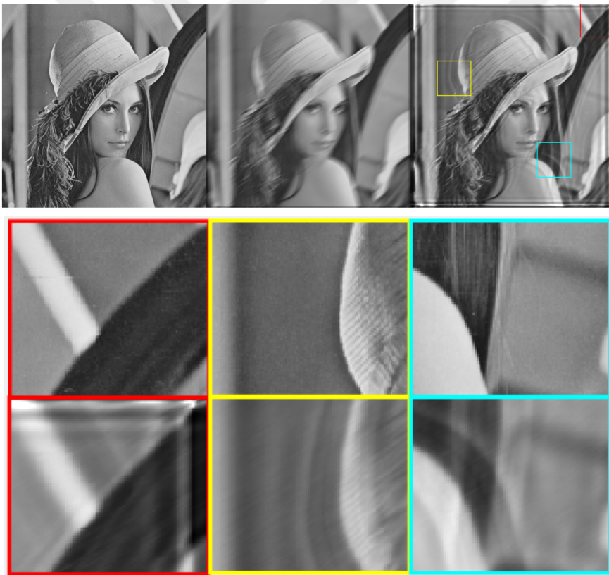
Figure 3.5: Original, blurred, and deblurred images are given at the top. Colored boxes from original and blurred ones are magnified in second and third rows respectively.
