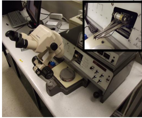
Figure 3.7: West bond wedge bonder. The inset shows the needle and the gold thread.
