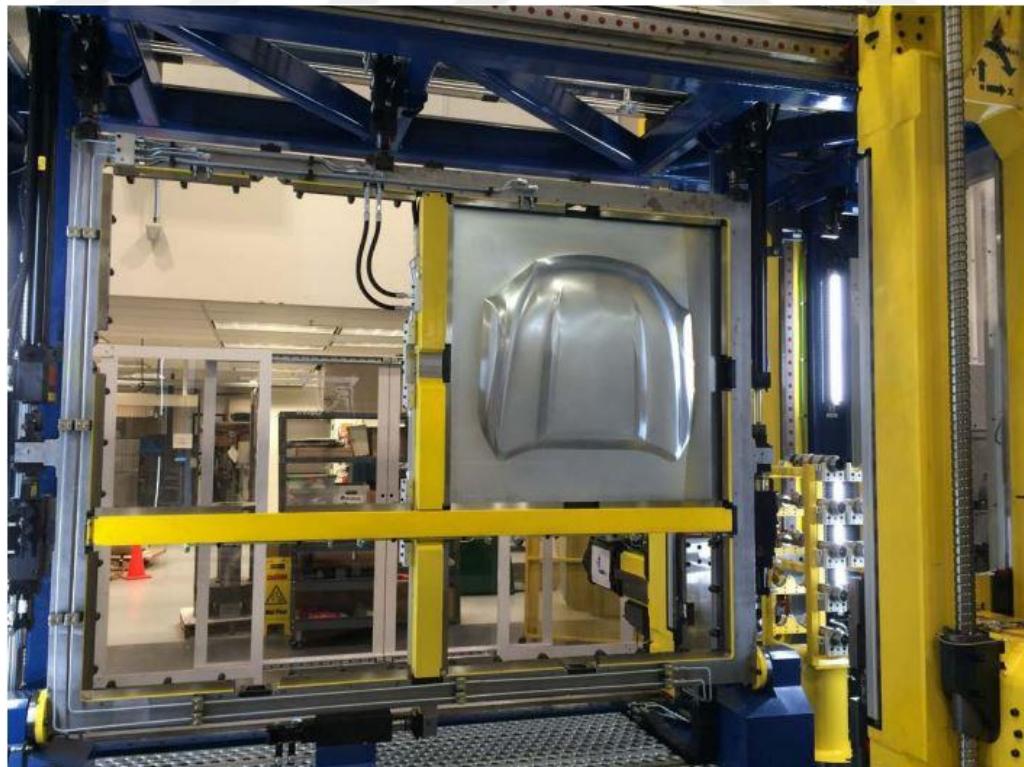
Figure 1.5: Rapid Freeform Sheet Metal Forming Technology (RAFFT) Machine producing a 0.4 scale Mustang hood in Ford Motor Co [43].
