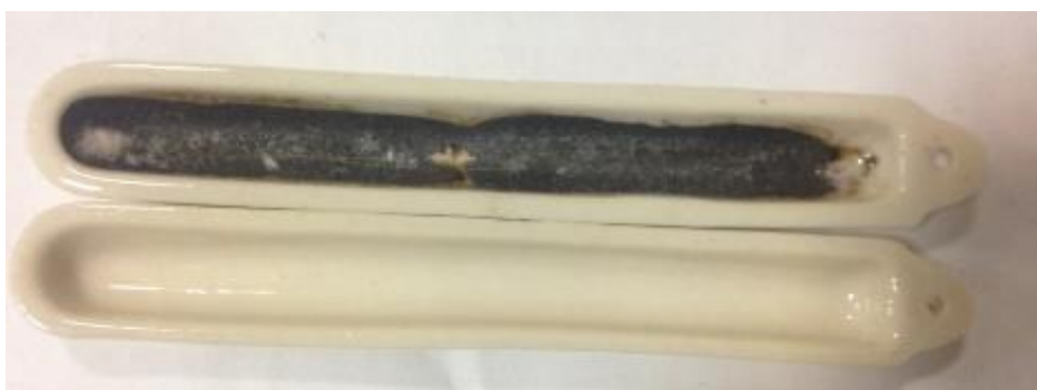
Figure 5.55. Ceramic cartridge before and after experiment of SCFM (6473)
