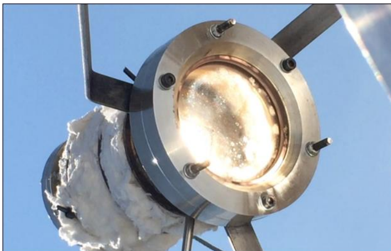
Figure 5.76. Solar reactor during the reforming operation
