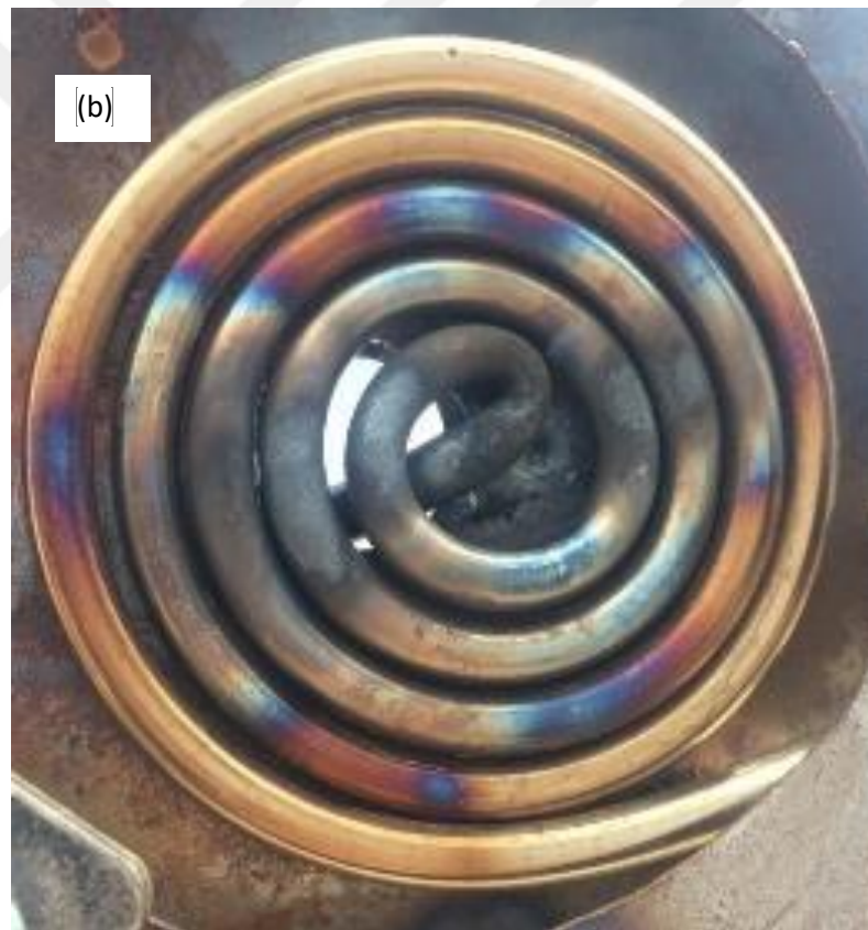
Figure 5.73. The variation of air temperature with respect to solar irradiation (a) and the spiral tubing after the air heating experiments (b)
