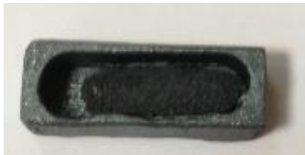
Figure 5.51. 316 stainless steel cartridge with SCFM (6473) after experiment
