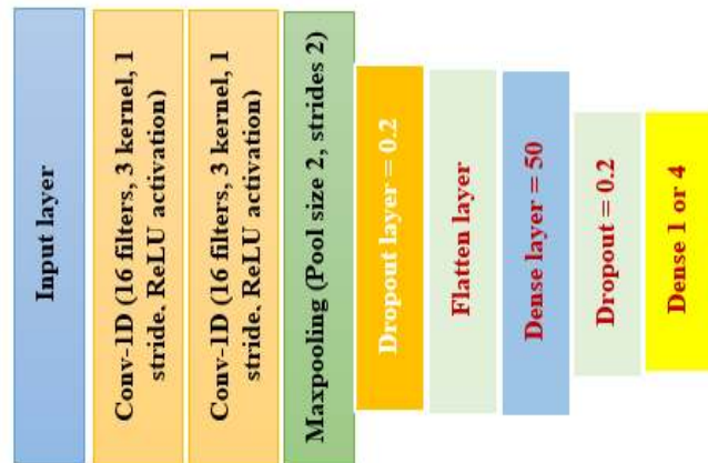
Figure 3.11. The 1D CNN architecture is used in this thesis
