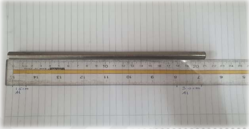
Picture 7.2. Iron sheath with \text{Mg} + 2\text{B} powder inside.
