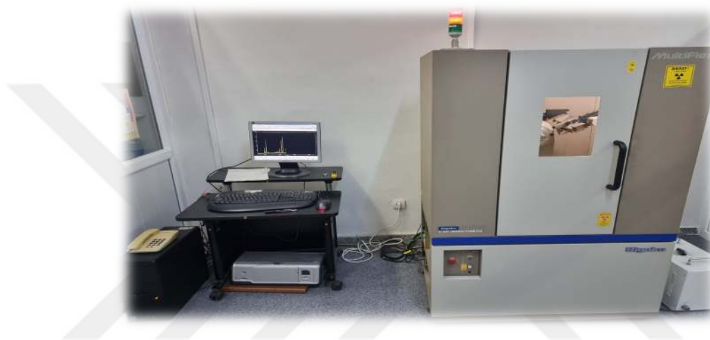
Picture 7.7. X-ray diffractometer for crystal structure analysis.
