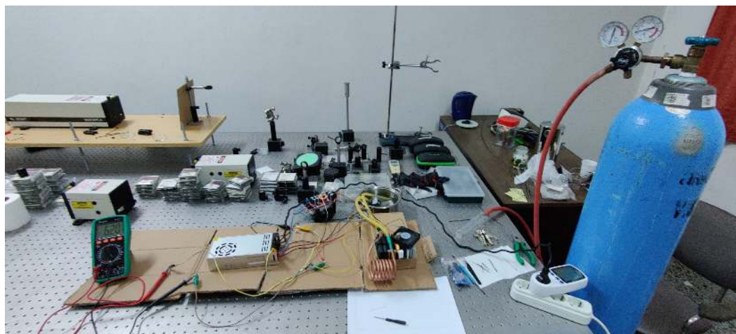
Picture 7.5. 1 kW induction heating system.
