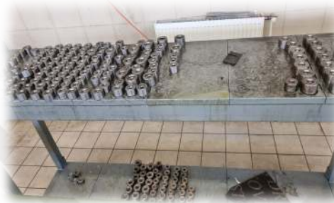
c) Tungsten Carbide Dies (inner diameters from 0.5 mm to 15 mm)
