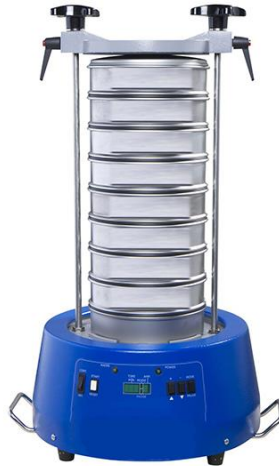
Figure 3.2 Sieve Shaker Machine
