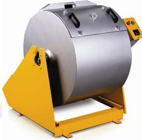
Figure 3.3 Los Angeles Abrasion Test Machine
