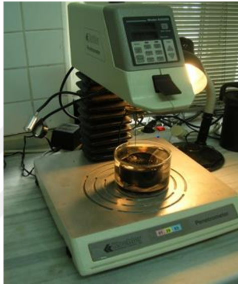
Figure 3.4 Penetration Testing Machine
