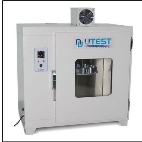
Figure 3.6 Thin film oven test machine
