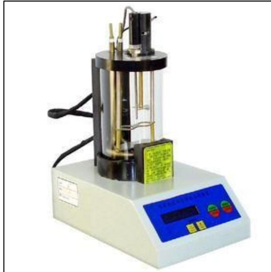
Figure 3.5 Automatic softening point device
