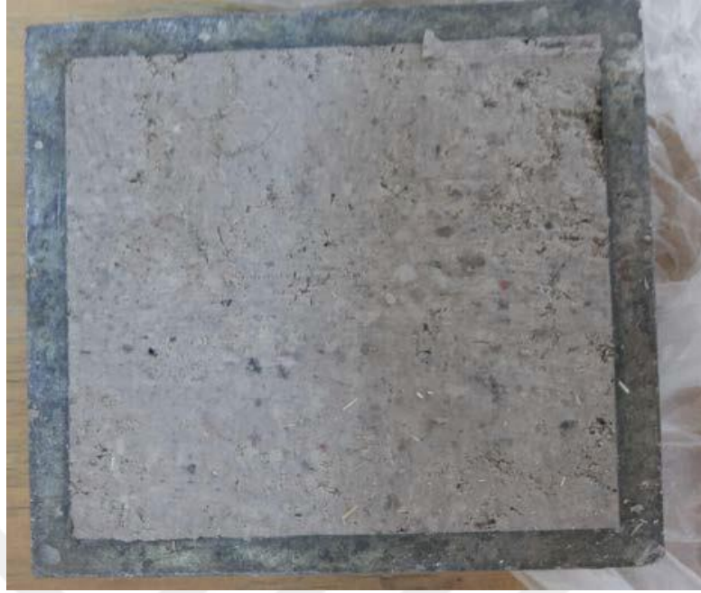
Figure 3.7 The soil samples in shear box
