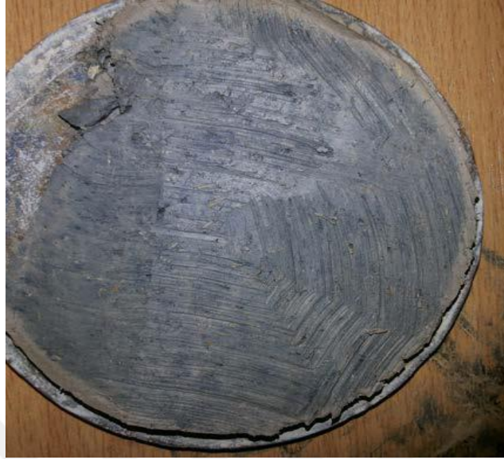
Figure 3.8 The soil testers in the ring of the unification apparatus
