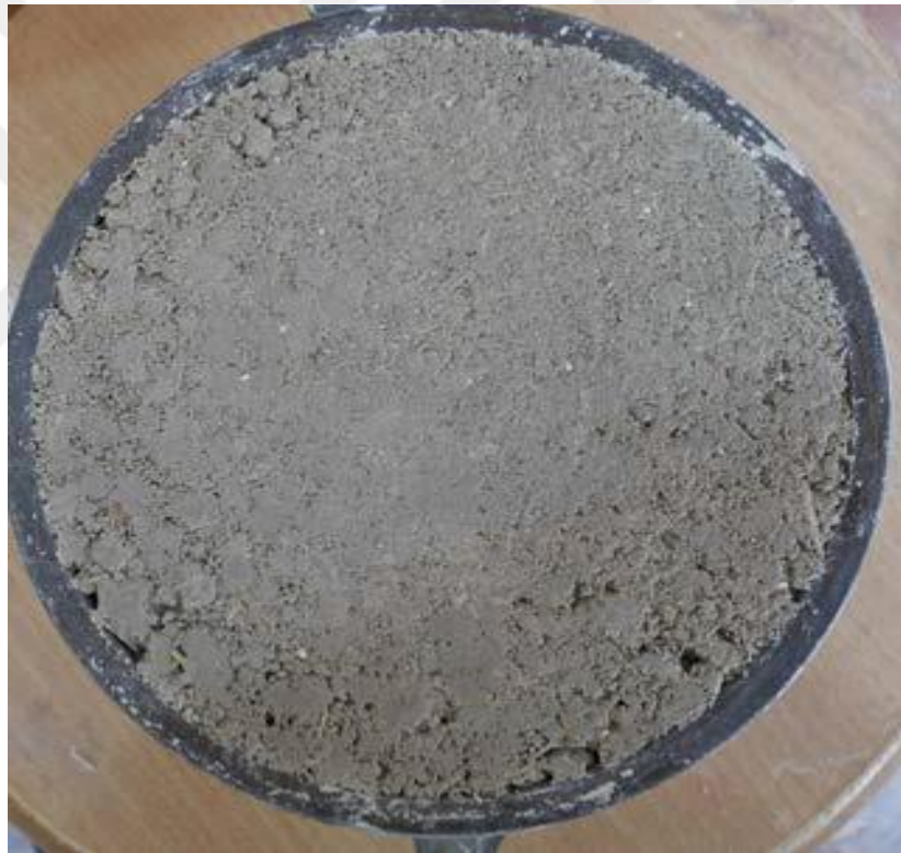
Figure 3.6 The soil samples compacted
