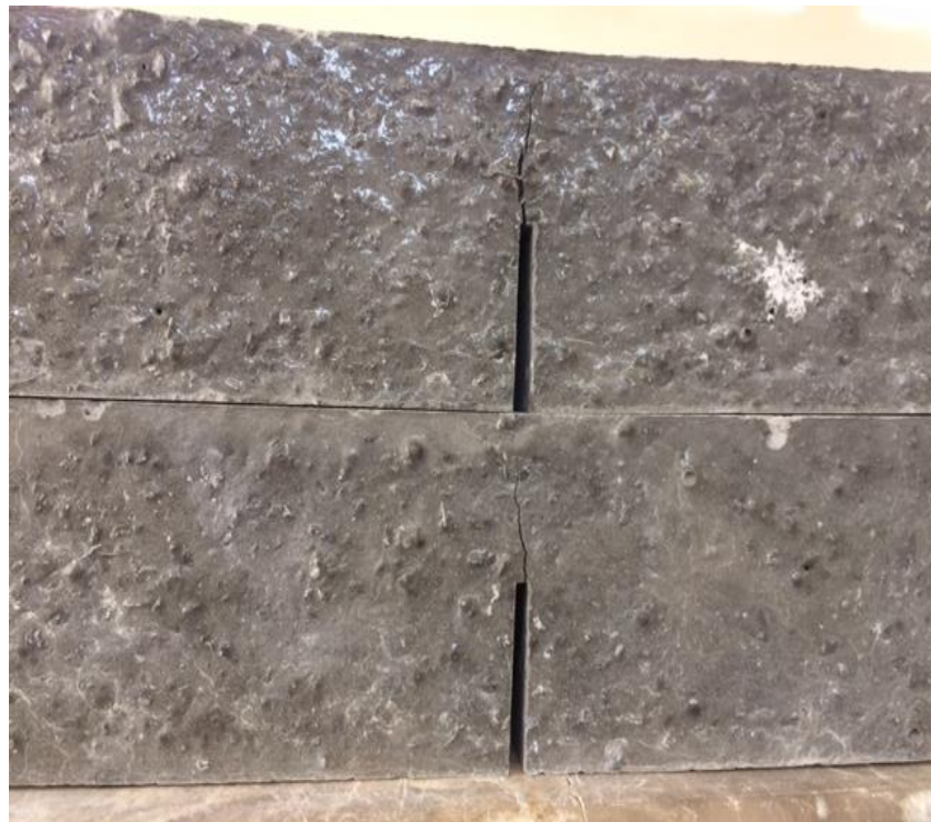
Figure 5.16: Failure Mode of Notched Flexural Specimens
