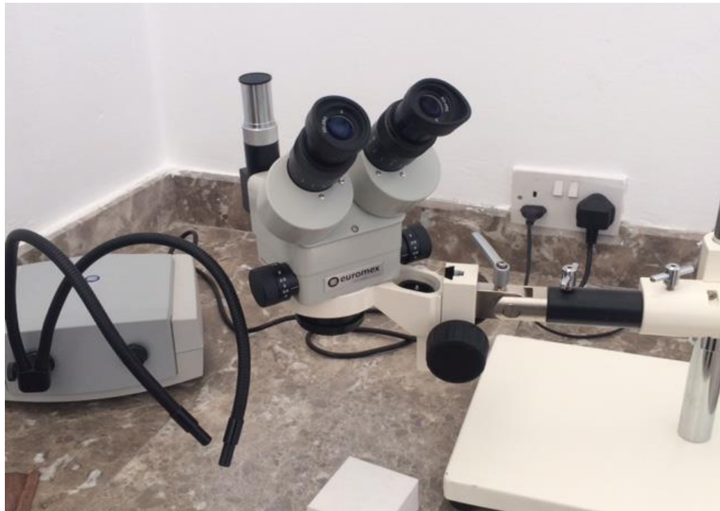
Figure 4.4: Optical Stereomicroscope used in this Study
