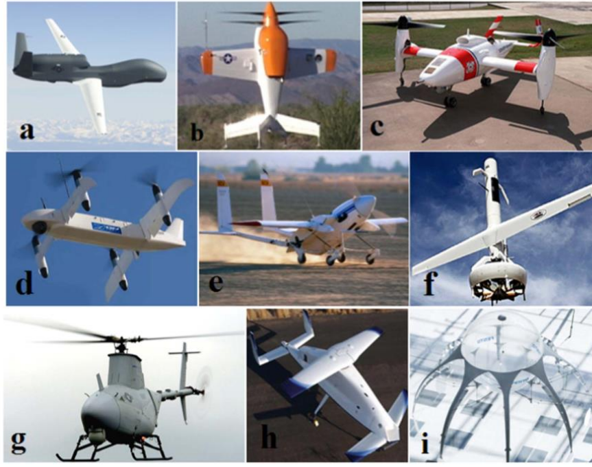
Şekil 2.5 Farklı dron tipleri, (a) HTOL, (b) VTOL, (c) tilt-rotor İHA, (d) tilt-kanat İHA, (e) tilt-iskelet İHA, (f) Kanallı fan İHA, (g) helikopter, (h) heli-kanatlı İHA, (i) Prototip İHA (Hassanalıan ve Abdelkefi 2017b).
