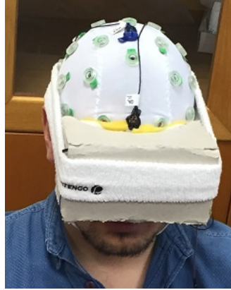
Figure 3.1: A photo of Do-It-Yourself (DIY) card-board VR headset
