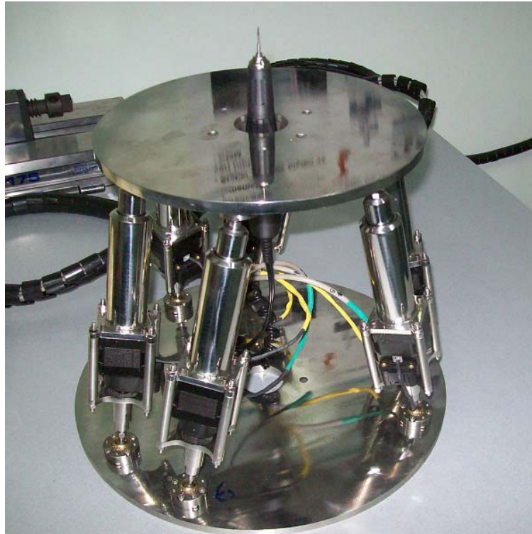
Figure 7.4 Hexapod assembly with backlash solution.
