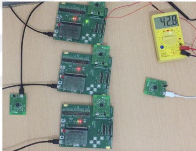
Figure 5.13. Measuring drawn current
