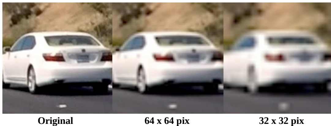
Figure 3.65. Scaling down the resolution of the image by using OpenCV.
