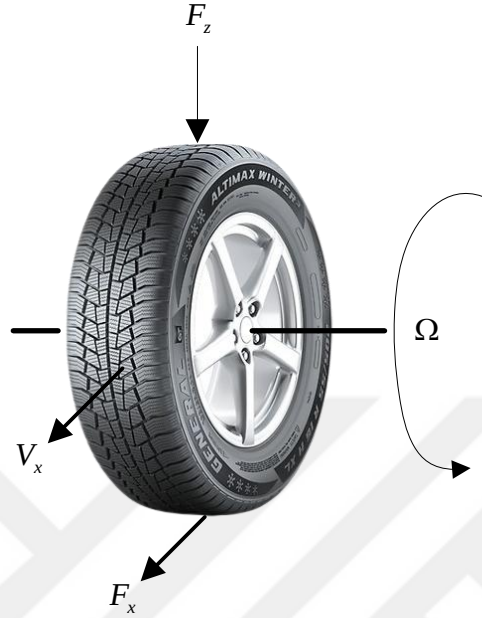
Figure 3.33. The forces affecting the tire.
