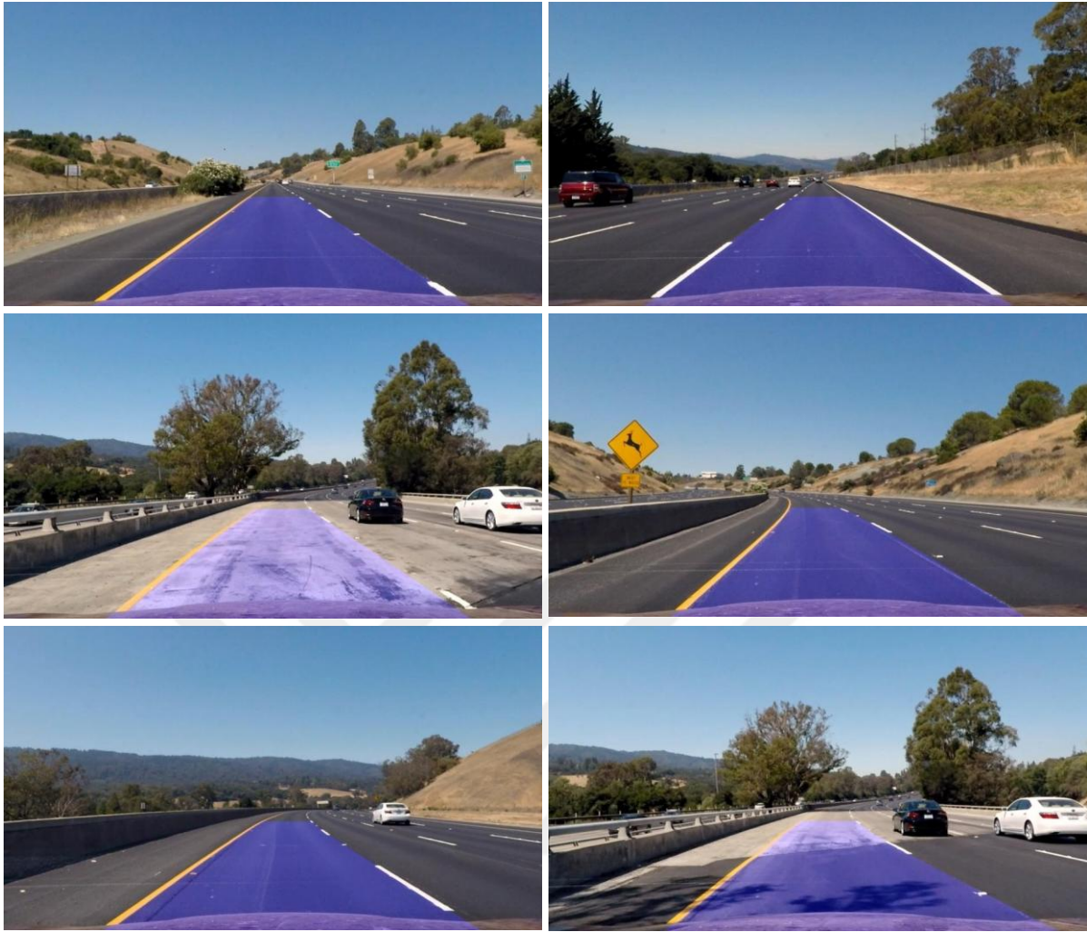
Figure 4.38. The lines detection in the various road images.
