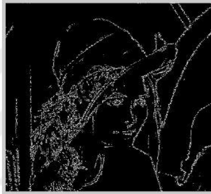
Figure 2.16. Image after applying Sobel operator [33]
