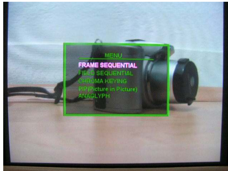
Figure 6.25 Menu interface at the output of the FPGA
