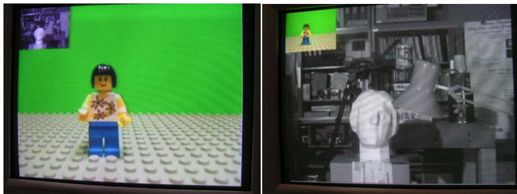
Figure 6.18 PIP application result at the output of the FPGA
