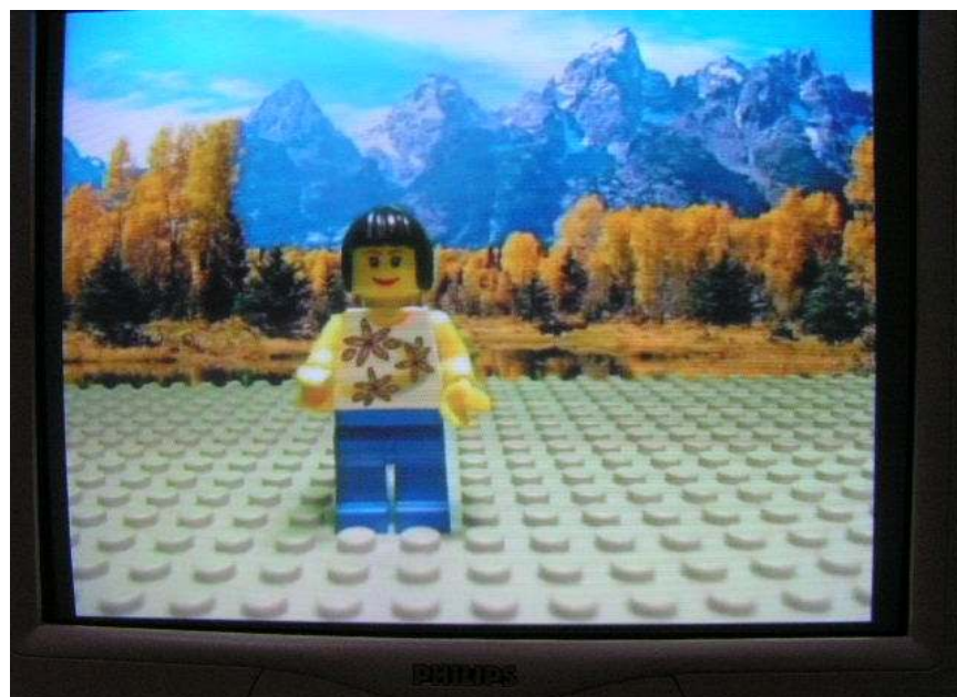
Figure 6.10 Chroma keying result at the output of the FPGA
