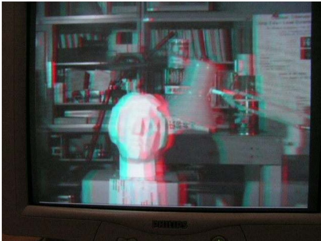
Figure 6.14 Anaglyph video result at the output of the FPGA
