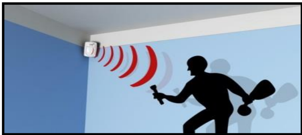
Figure 5.1. Perimeter detection through motion sensor
