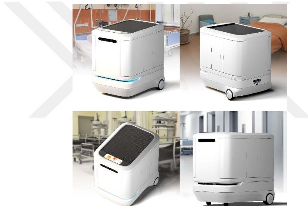
Figure 2.1: (Color online) A service robot designed by FDATA for delivering supplies efficiently and safely in the hospital [Fdata Co., 2025].
