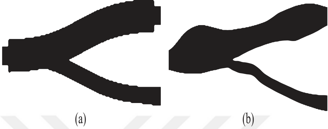
Figure 3.9: 90%:10% power splitter with design region area of 7.0 \times 7.0 \mu\text{m}^2 and filter radius of 1.25 \mu\text{m} : (a) Initial guess geometry, (b) Optimized 90%:10% power splitter.
