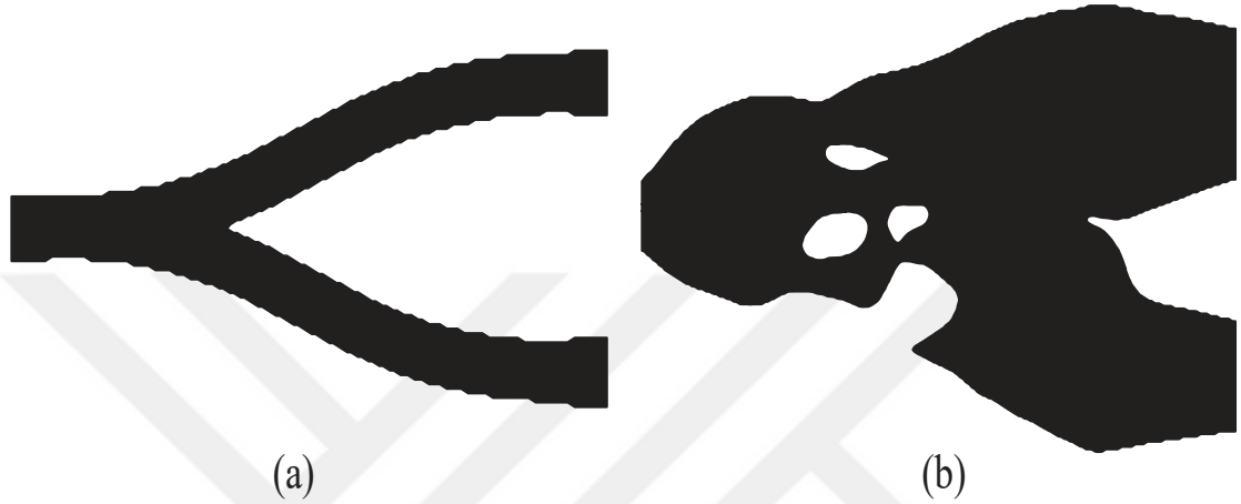
Figure 3.2: 90%:10% power splitter with design region area of 6.0 \times 6.0 \mu\text{m}^2 and filter radius of 1.0 \mu\text{m} : (a) Initial guess geometry, (b) 90%:10% power splitter.
