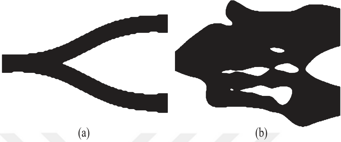
Figure 3.5: 90%:10% power splitter with design region area of 6.0 \times 5.0 \mu\text{m}^2 and filter radius of 1.0 \mu\text{m} : (a) Initial guess geometry, (b) Optimized 90%:10% power splitter.
