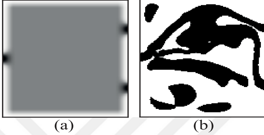
Figure 3.26: Photonic spectral filter with a design area of 6 \times 7.2 \mu\text{m}^2 , the radius and penalty radius of 250 nm : (a) Initial guess, (b) Optimized spectral filter.
