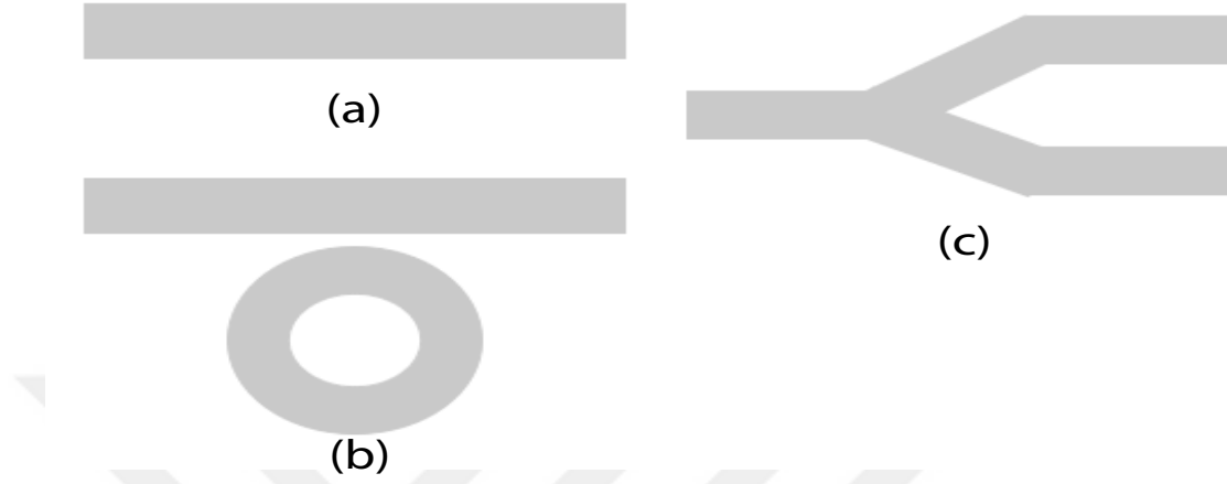
Figure 1.1: (a) Initial guess for straight waveguide for specific functionality, (b) Initial guess for ring resonator, (c) Initial guess for 50%:50% power splitter
