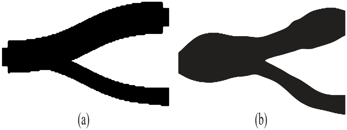
Figure 3.14: 90%:10% power splitter with design region area of 8.0 \times 6.0 \mu\text{m}^2 and filter radius of 1.5 \mu\text{m} : (a) Initial guess geometry, (b) Optimized 90%:10% power splitter.
