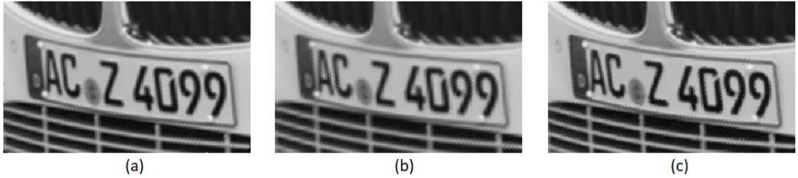
Figure 4.12. Reconstructed 'plate' image using (a) cubic, (b) IDW and (c) IDW_{sel}
