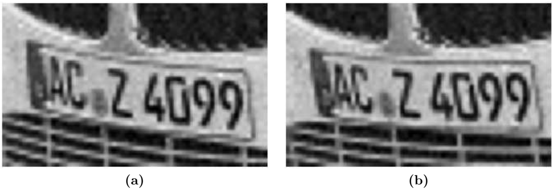
Figure 2.18. Synthetically generated LR images of a car license plate with additive Gaussian noise
