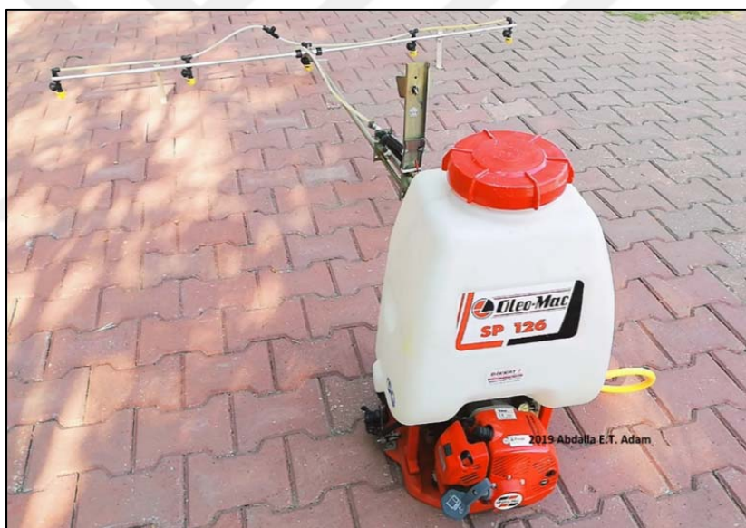
Figure 3.12. A motorized backpack sprayer used for herbicide application on dwarf mesquite [ Prosopis farcta (Banks & Sol.) F.J. Mac.] during the field experiments.
