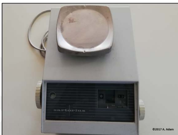
Figure 3.13. A sensitive scale used for measuring the fresh and dry weights of plant harvested from both greenhouse and field studies.
