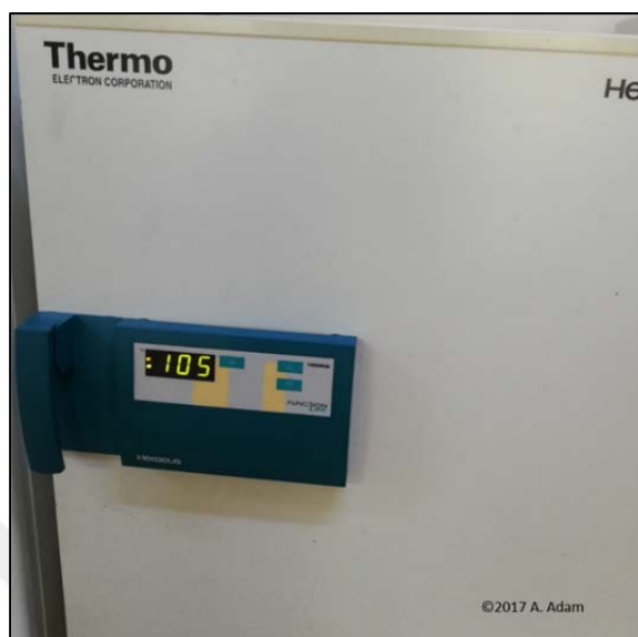
Figure 3.14. Drying oven used for drying plant shoots.
