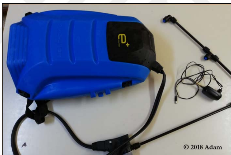
Figure 3.11. A rechargeable electric battery sprayer (Matabi) used for herbicide application in the greenhouse experiments.
