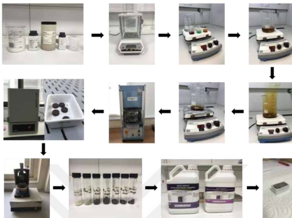
Figure 3.7. Step-by-steps from nanomaterial production to composite material production.
