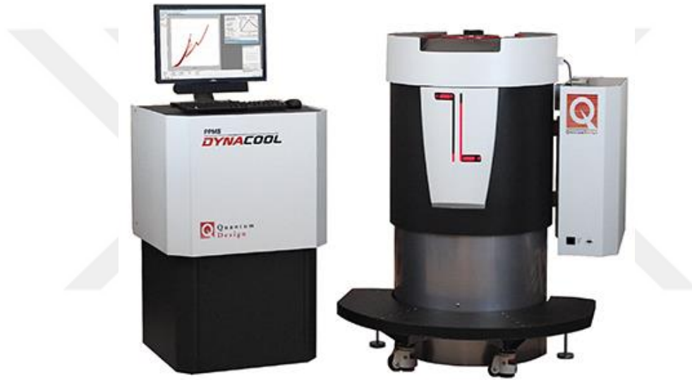
Figure 3.5. Quantum Design Dyna-Cool model Physical Property Measurement Sytem (PPMS).
