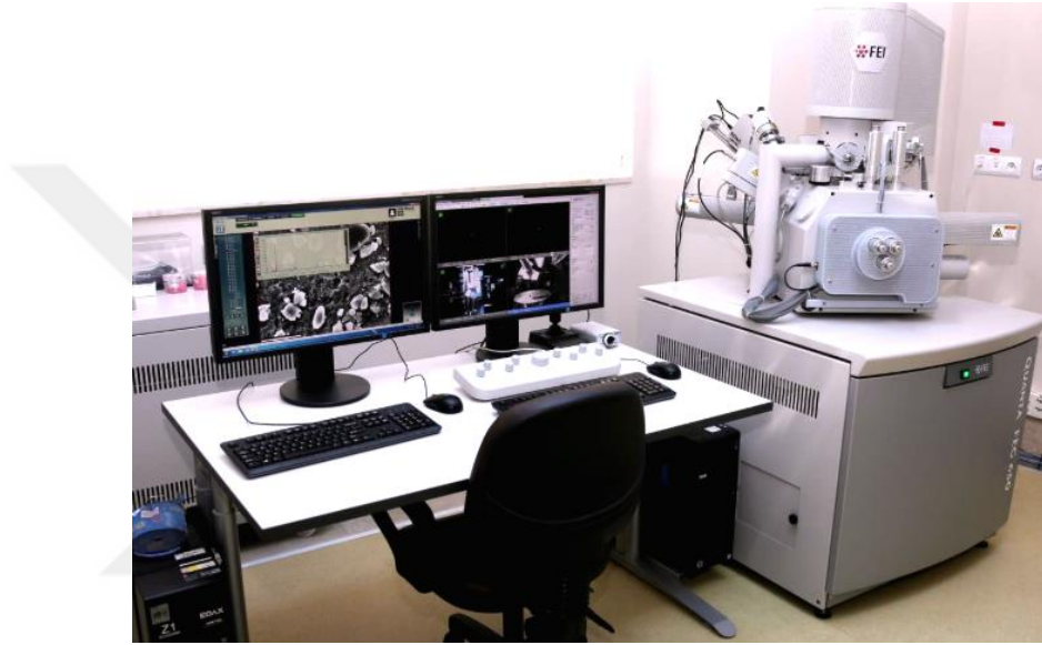
Figure 3.4. FEI Quanta FEG-650 type scanning electron microscope with EDS integrated.
