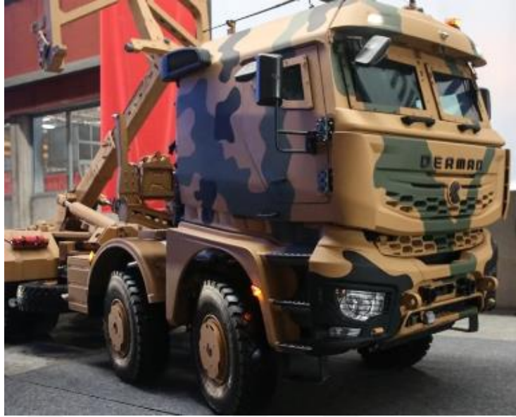
Figure 1.6. Vehicle cabin with ballistic protection provided by armor steel (Koluman, Derman).
