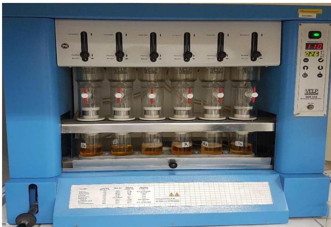
Figure 3.8: Soxhlet system used for crude lipid analysis in the Fish Nutrition Laboratory at Istanbul University.
