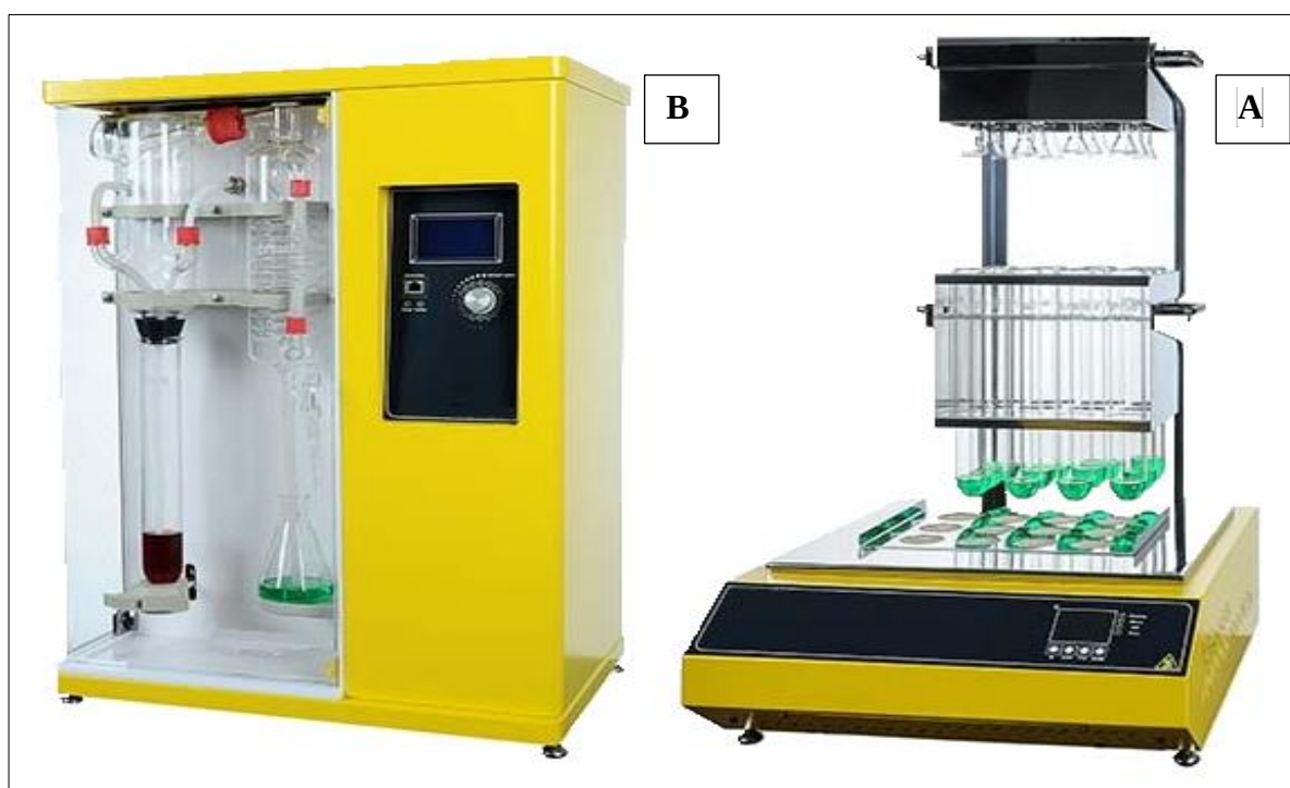
Figure 3.7: Digestion unit (A) and distillation unit (B) of the Kjeldahl system used for crude protein analysis in the Fish Nutrition Laboratory at Istanbul University.
