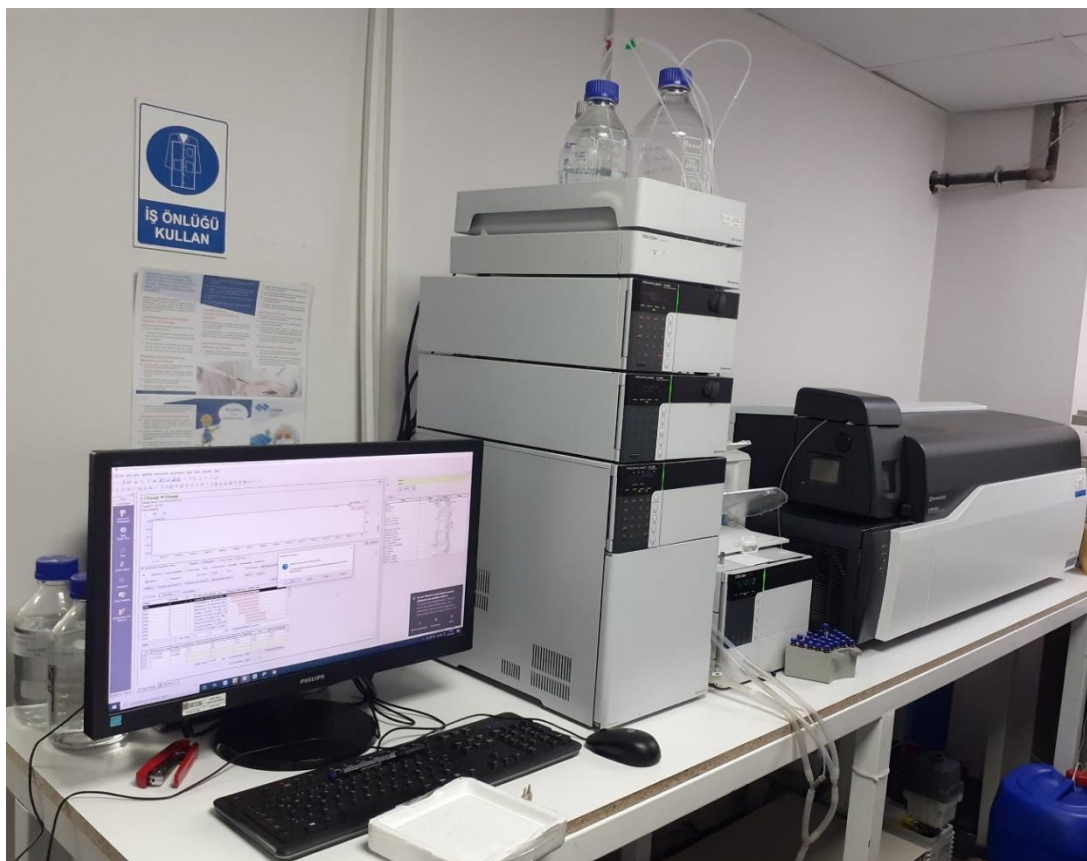
Figure 3.9: Liquid Chromatography Mass Spectrometer system (LCMS 8050) used for the analysis of amino acids in the GTS Test Laboratories-Department of Chemistry.
