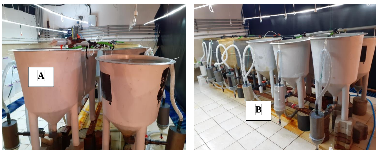
Figure 3.3: Cylinder-conical tanks used in the collection of fish feces during the experiment. (A) cylindro-conical experimental tanks (B) fecal collection system.
