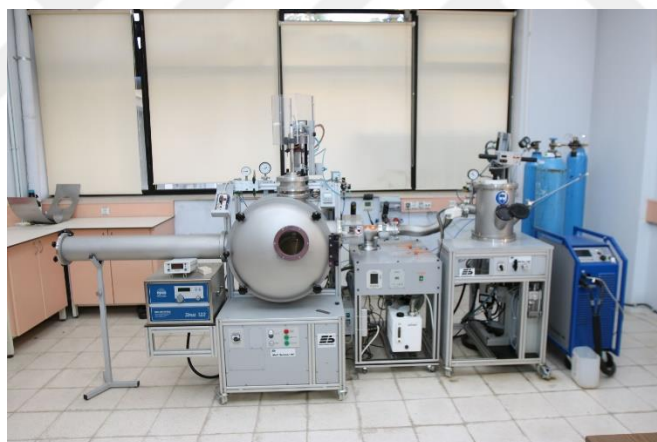
Figure 2.20 Arc-melter for preparing metallic alloy with atmosphere control system.
