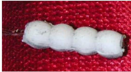
Figure 2.6 The prototype of earthworm robot [27].
