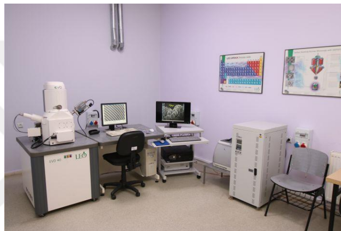
Figure 2.22 Scanning Electron Microscopy-Energy Dispersive X-ray Spectrometry (SEM-EDX).
