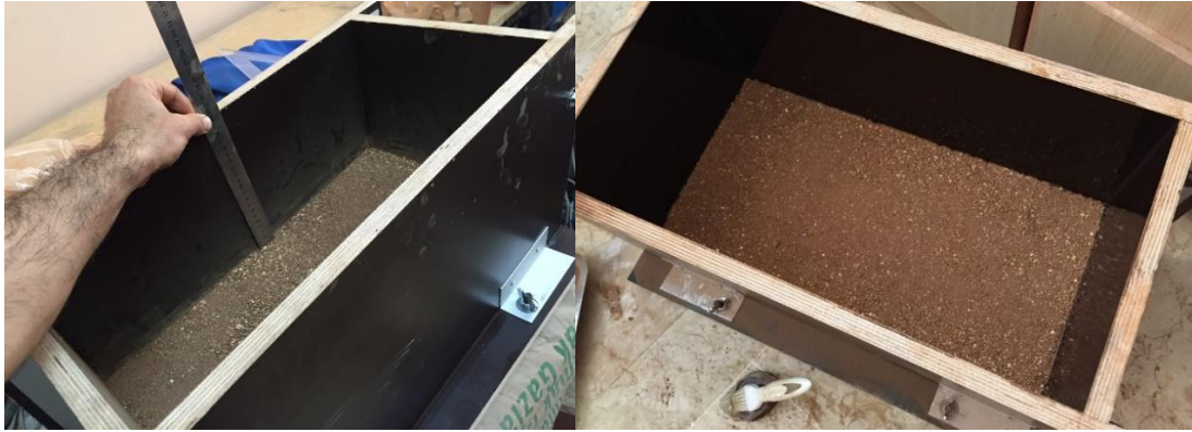
Figure 3.10 Fully compacted layer of clay.
