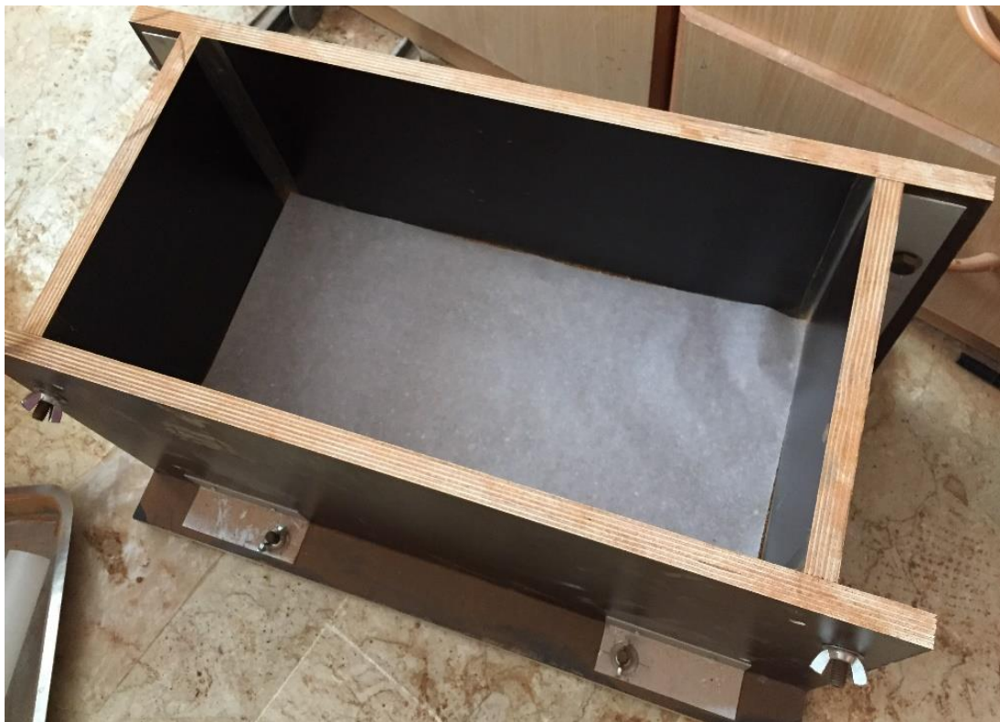
Figure 3.11 Anti-adhesion sheet added before oiling the mold.
