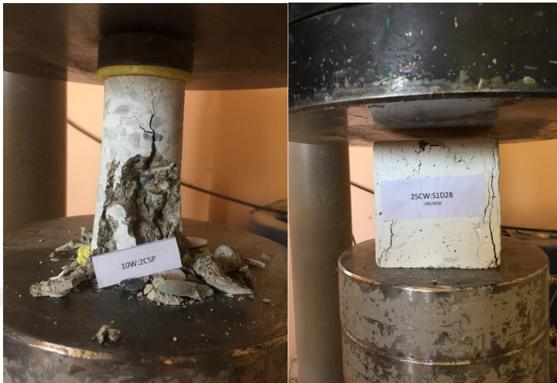
Figure 4.1 Samples during compressive strength test.
