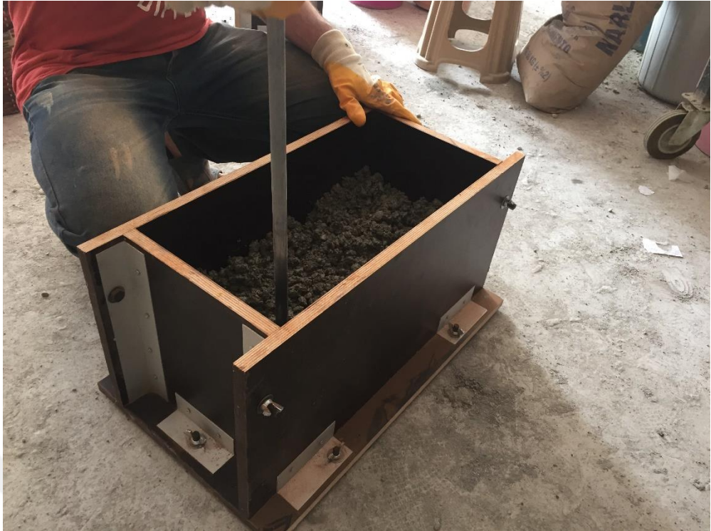
Figure 3.14 During the casting process.
