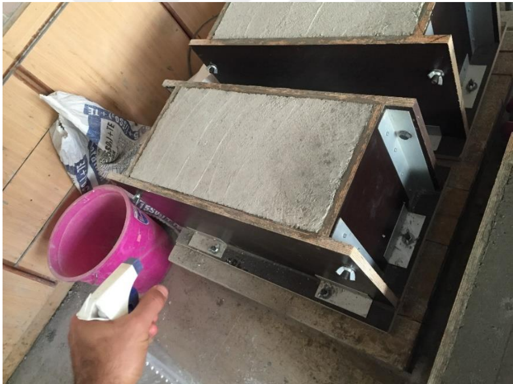
Figure 3.15 The Curing method that used in this study.
