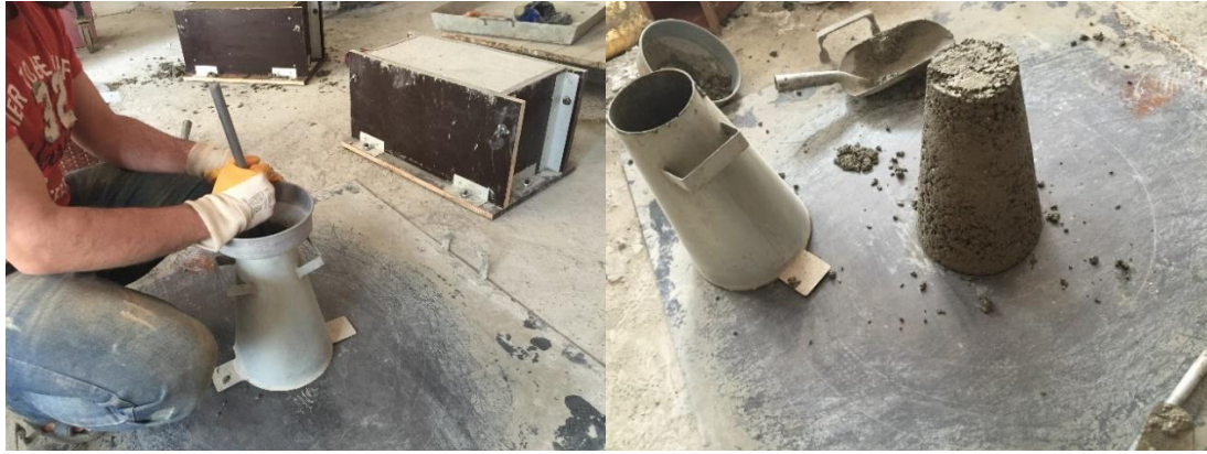
Figure 3.18 Slump test method procedure.
