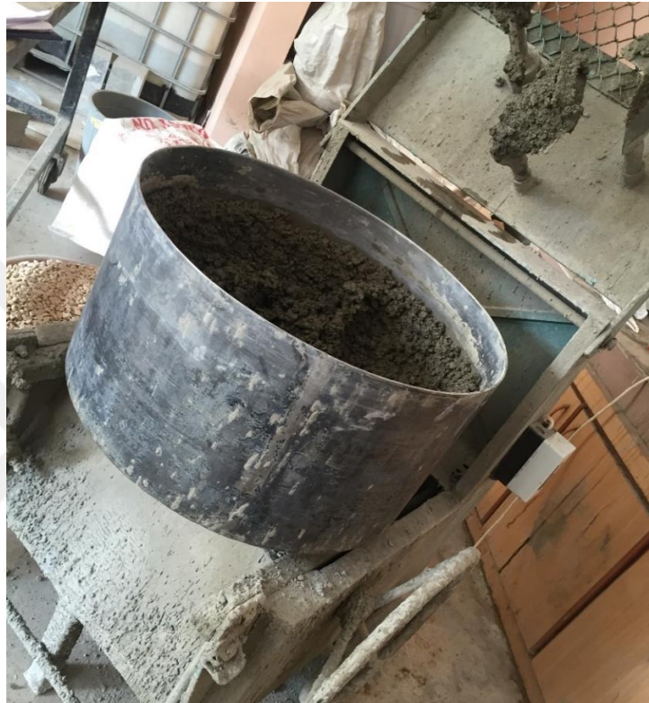
Figure 3.13 Power-driven revolving pan mixer used in this study.
