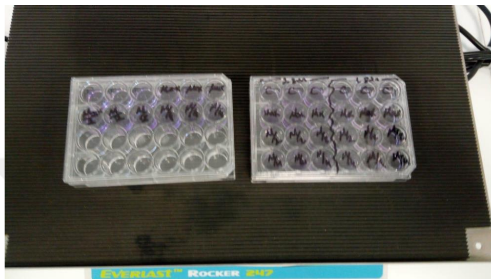
Figure 3.2. Dissolving samples. Samples were shaken on Everlast Rocker 247 after treatment with isopropanol.
