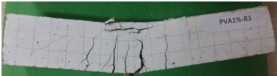
Figure 4.6 Sample of marking the tested beam.
