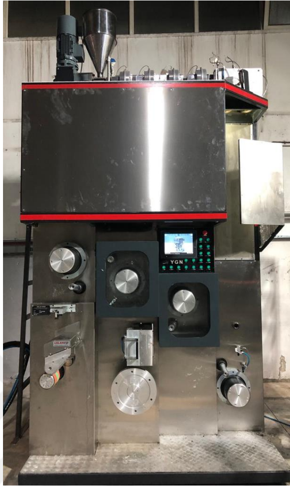
Figure 4.2 Laboratory type melt spinning machine used for the production of frc-PET filaments
