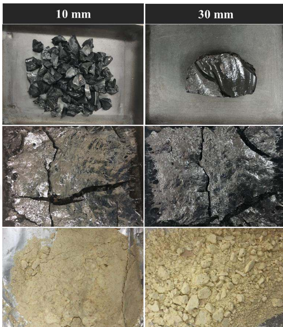
Figure 3.13 Carbonized materials and chemicals obtained from the carbonization of 10 mm and 30 mm d -PET
