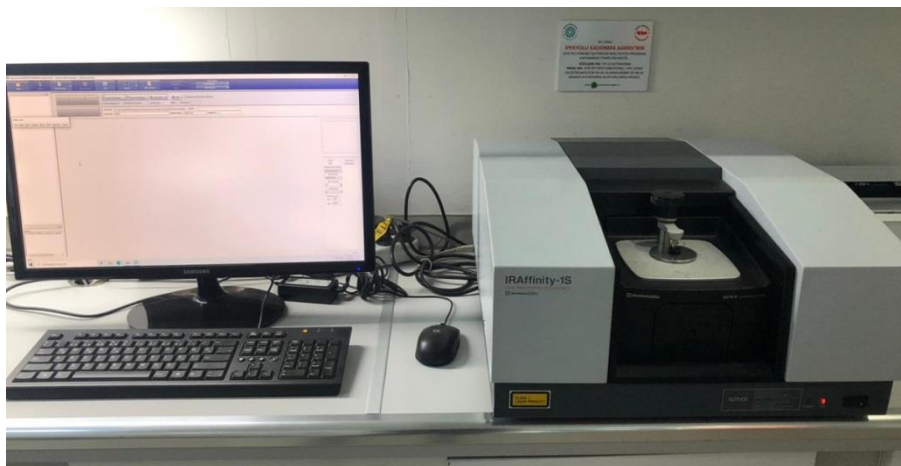
Figure 3.4 SHIMADZU IRAffinity-1S Fourier-transform infrared spectrometer
