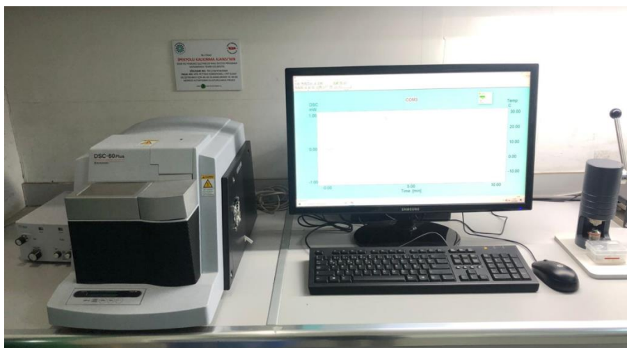
Figure 3.2 SHIMADZU DSC-60 Plus differential scanning calorimeter
