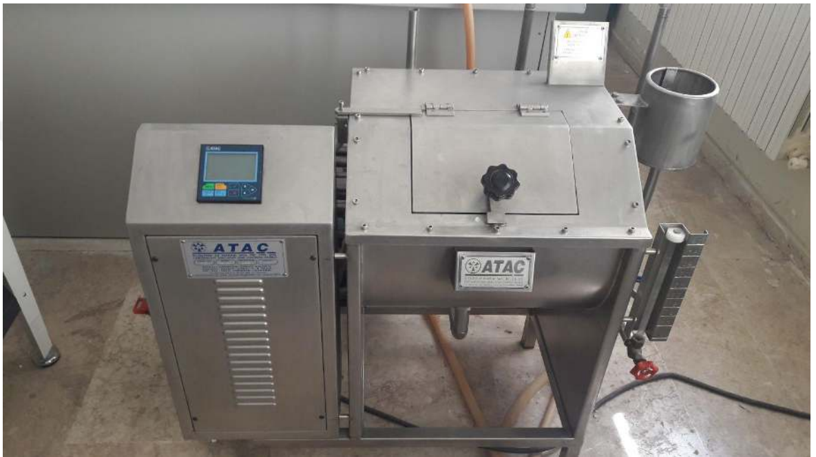
Figure 2.8 ATAC Dyeing Machine
