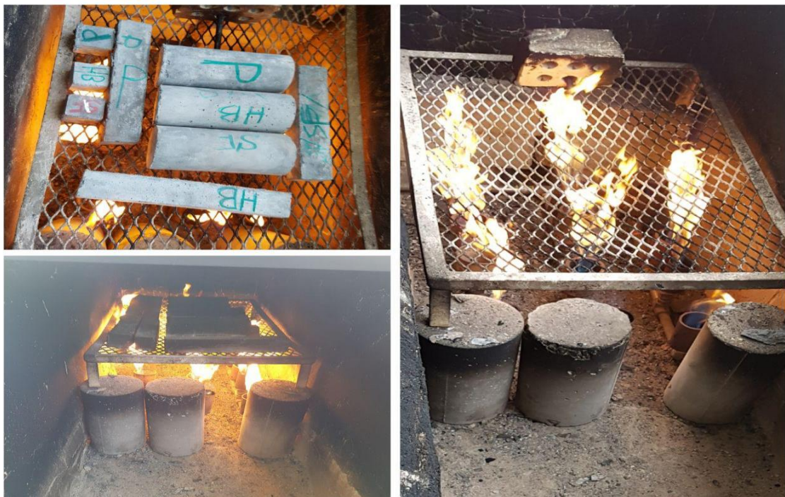
Figure 3.19: The Burning Process for Samples ( Cube, Cylinder, Prism).
