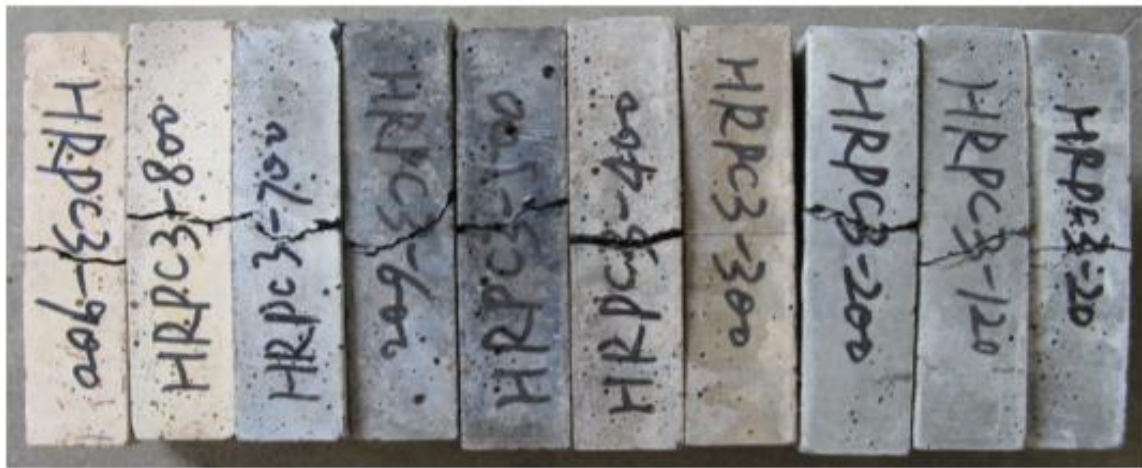
Figure 2.6: HRPC Flexural Failure's Type After Extreme Temps, Haiyan (2016).
