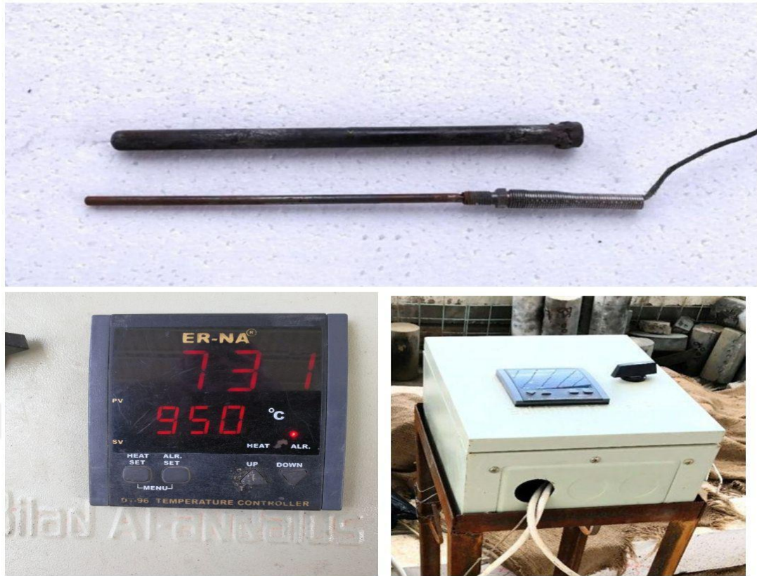
Figure 3.15: Specifics of Thermocouple and Digital Gage.
