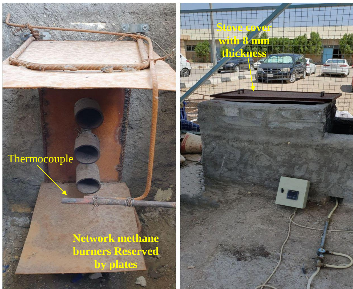
Figure 3.14: Specifics About the Stove and its Network of Burners' Methane.
