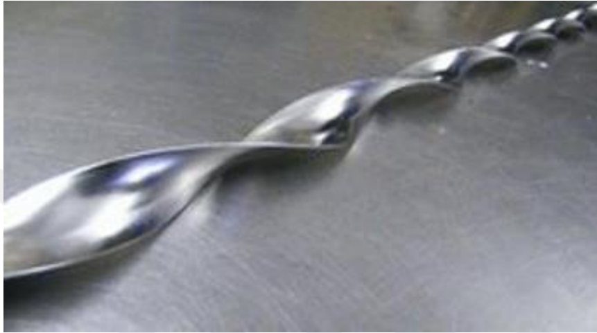
Figure 1.2. Full length twisted tape as a passive technique (Chintan et al., 2012)
