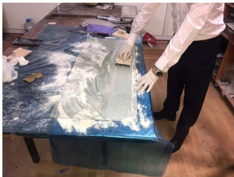
Figure 3.10 Surface treatment procedure used to prepare substrate surfaces
